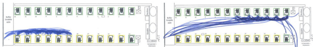
Figure 4. A spaghetti diagram was performed for 1 h in the branding sector, considering the use of carts (left) and baskets (right).
