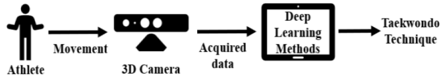
Figure 13. Deep-learning methods testing system diagram.
