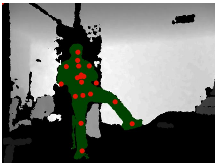
Figure 5. Identification of skeletal joints with Nuitrack™ middleware, via depth sensor.
