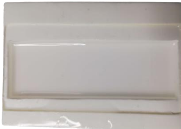
Figure 4.6 – Polyurethane mould for the staggered herringbone micromixer
