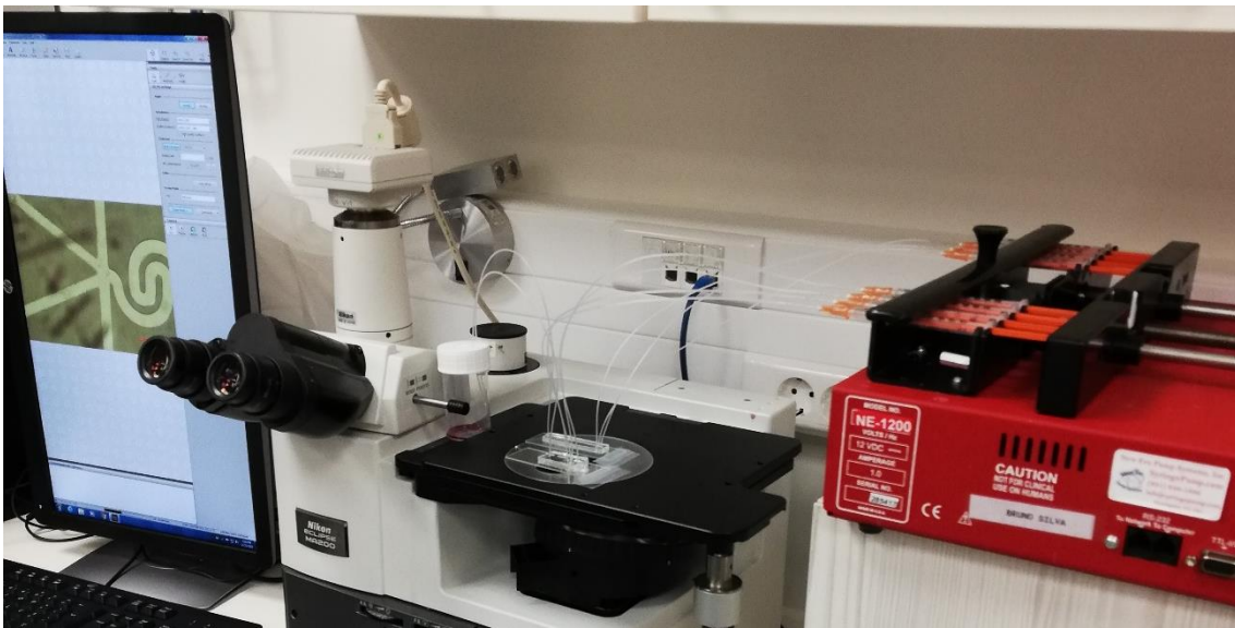
Figure S.6 – Pumping mechanism setup. The syringe pump is adjusted manually to program de flow rate, the amount of volume pumped, and the diameter of the syringes inserted. Tubing and connectors are used to connect the syringes to the device that is on top of the microscope. A computer with the appropriate software gives us a real-time illustration of what is occurring during the pumping.
