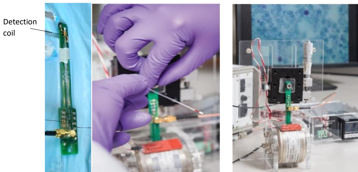
Figure 8: Bench-top setup NMR system, with a PCB (printed circuit board) probe, a micro coil for sample detection. Capillaries are placed into the coil with the end containing concentrated iRBCs. Adapted from Peng et al. INL laboratory protocol, NMR setup with a capillary tube containing concentrated blood at one end.
