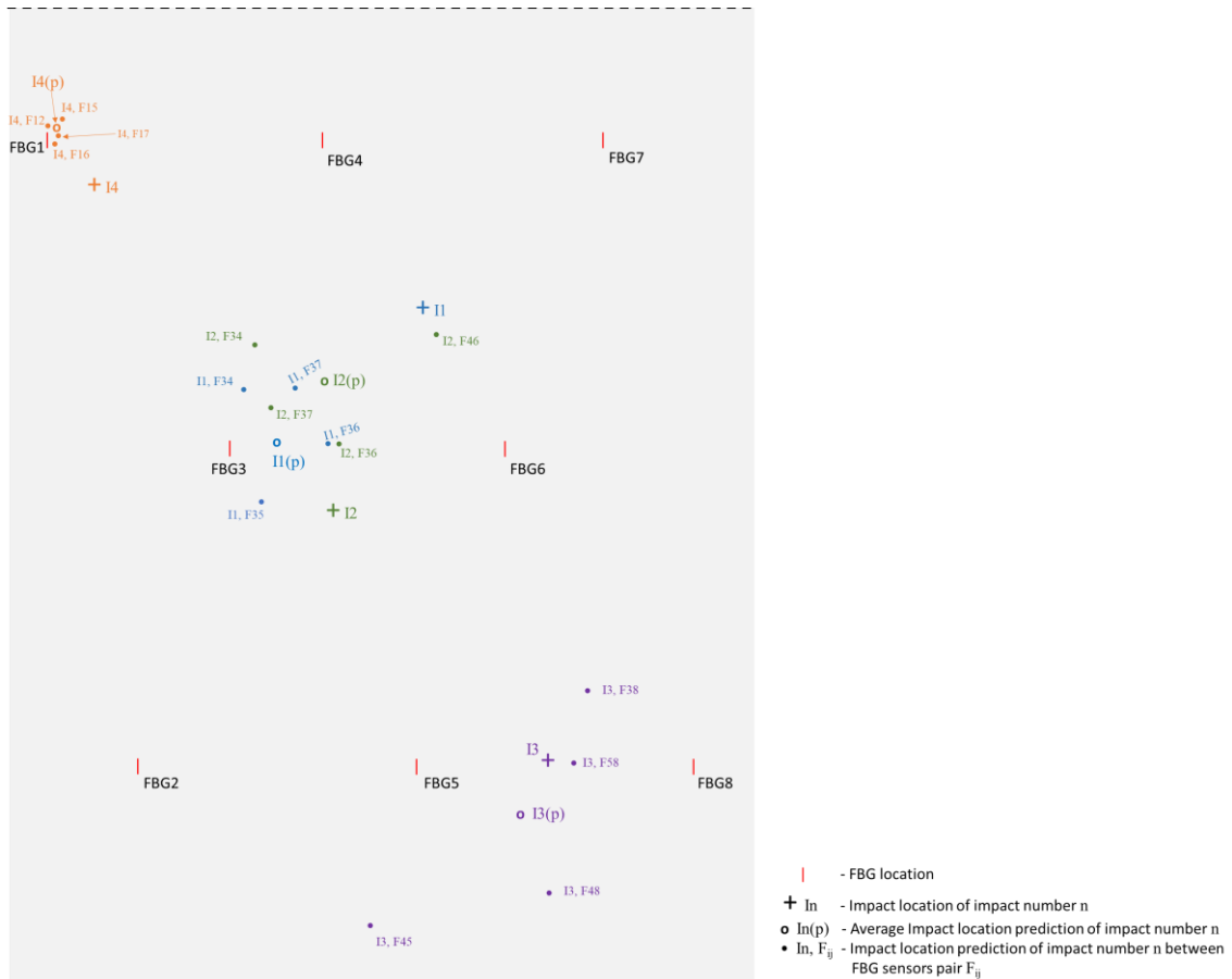
Figure 90: Real and predicted Impact locations on the flat projection of the COPV cylindrical region
