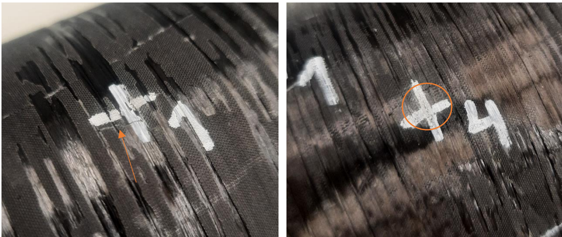
Figure 91: Barely visible impact damage on the COPV surface: (a) matrix crack and (b) small bump
