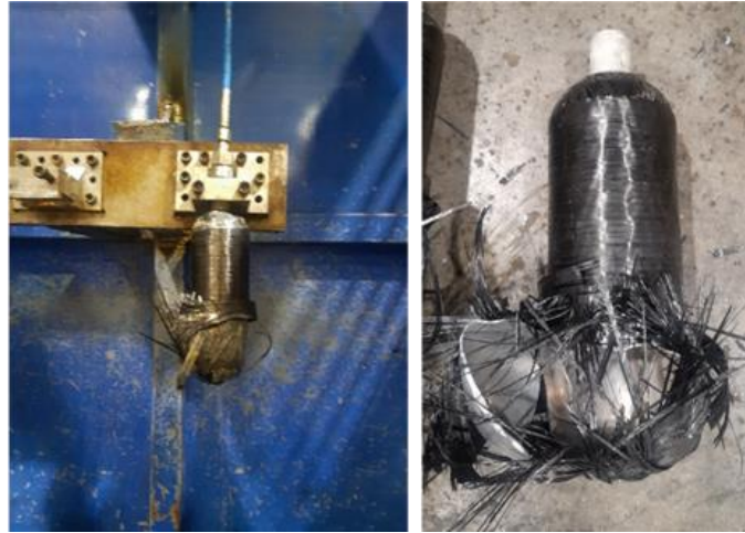
Figure 83: COPV after burst test
