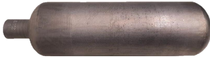
Figure 36: Picture of the 6061-T6 Aluminium liner
