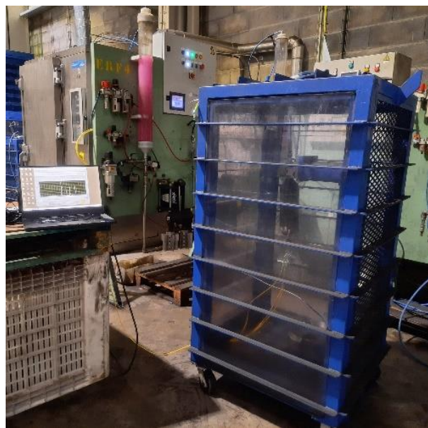
Figure 46: Cyclic pressure test and OF monitoring setup at Amtrol-Alfa
