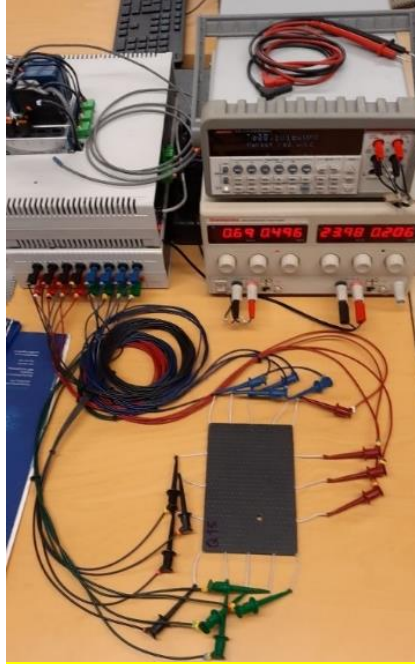
Figure 29: Electrical impedance tomography equipment
