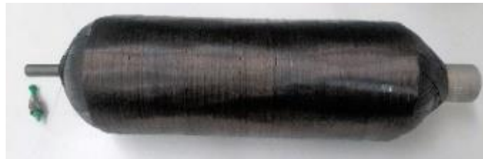
Figure 89: Smart COPV with embedded FBG sensors
