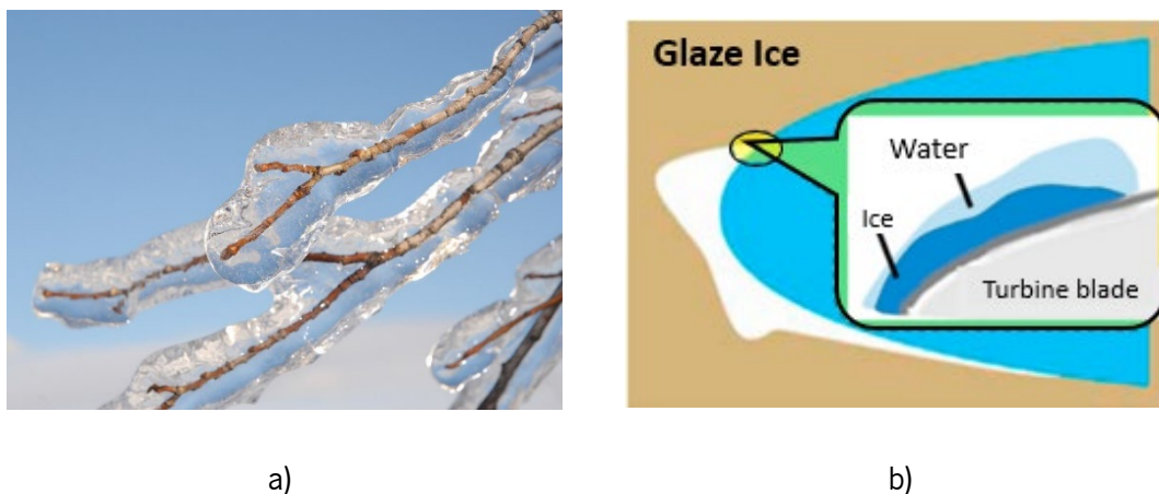
Figure 2.4 – a) Glaze ice [15]. b) Glaze ice accretion over wind turbine blades [14].
