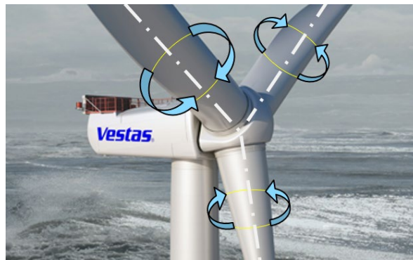
Figure 2.13 – Blade pitch control (adapted from [22]).
