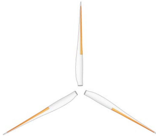
Figure 2.8 – Placement of the heating elements on the leading edges of the wind turbine blades [7].
