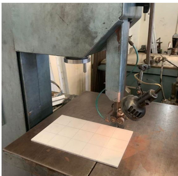
Figure 3.3 – Vertical band saw used to cut the blade samples.
