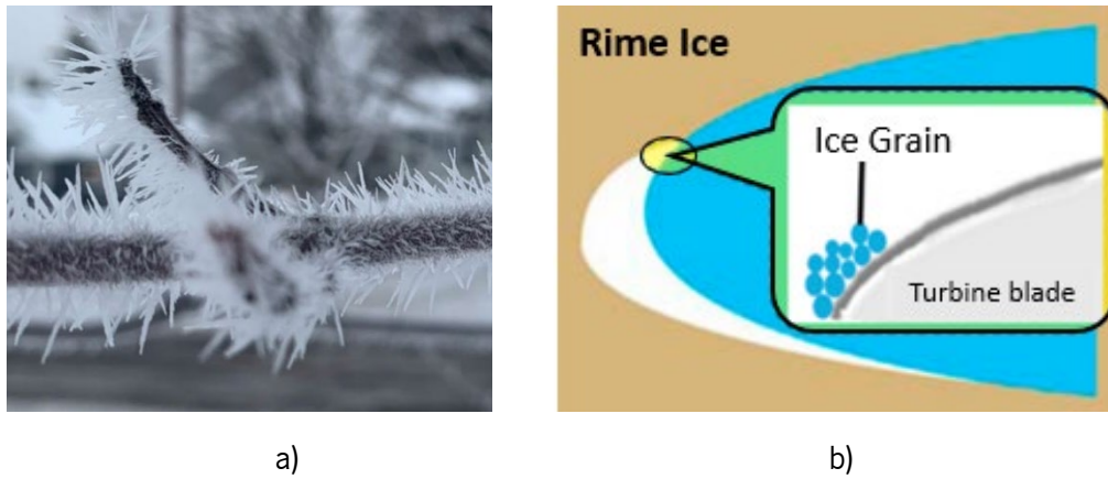
Figure 2.3 – a) Rime ice on a tree [13]. b) Rime ice accretion over wind turbine blades [14].
