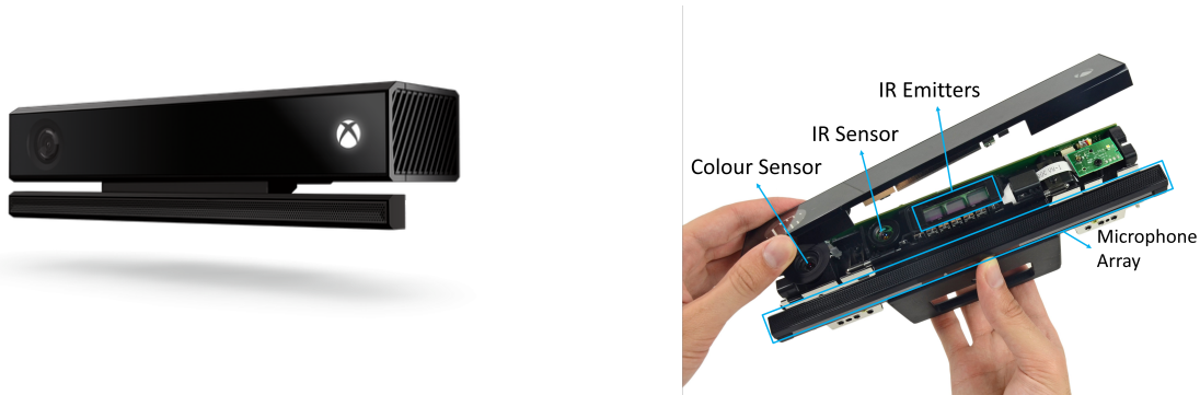
Figure 4.1: Microsoft Kinect v2 1 and its internal sensors 2
