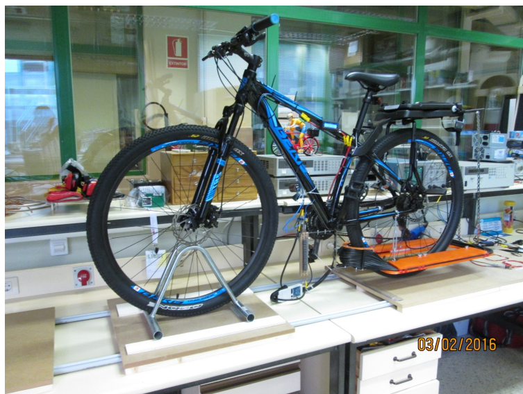
Figure 190: First test of the partially adapted e-bike on the energized primary coil.
