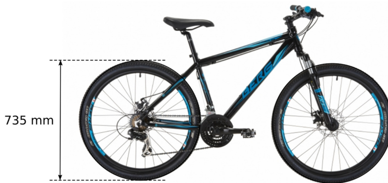
Figure 147: Bike model procured for adaption as a HIPLEV, a 29er with aluminum frame and wheels.
