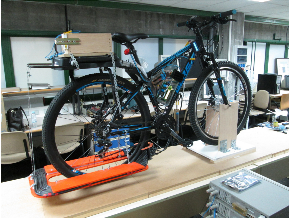
Figure 204: HIPLEV prototype on new all-wooden test workbench, shown with primary coil totally covered.
