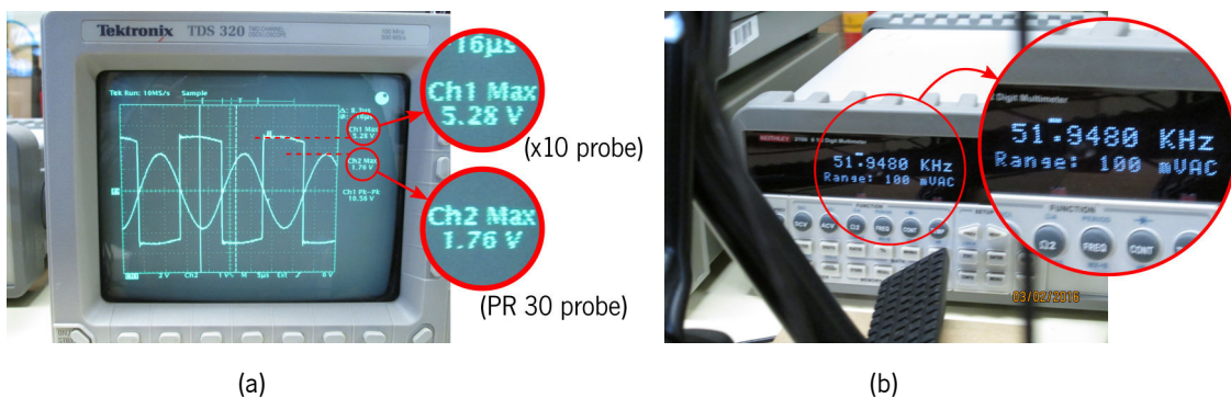
Figure 194: Photos of the other auxiliary instruments reading: (a) secondary coil current and secondary link voltage, which is the input to the diode bridge and (b) induction frequency.
