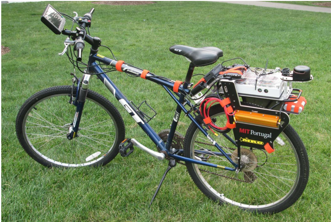
Figure 253: Electro-optical DIWPT evaluation system mounted on a regular bike.
