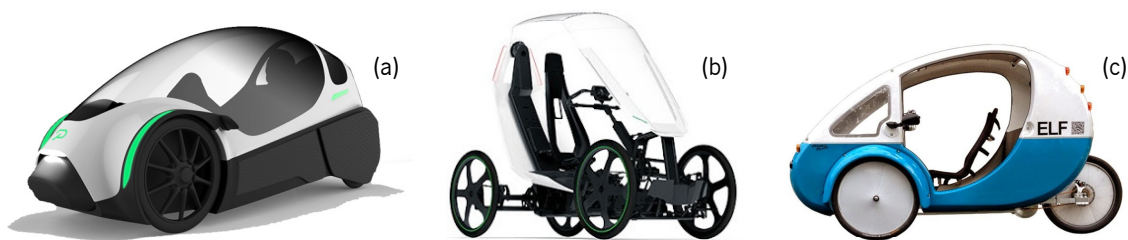
Figure 144: Examples of human-powered lightweight electric vehicles of recent design: (a) Sørensen's Podbike, (b) Schaeffler's Bio-Hybrid and (c) Organic Transit ELF.
