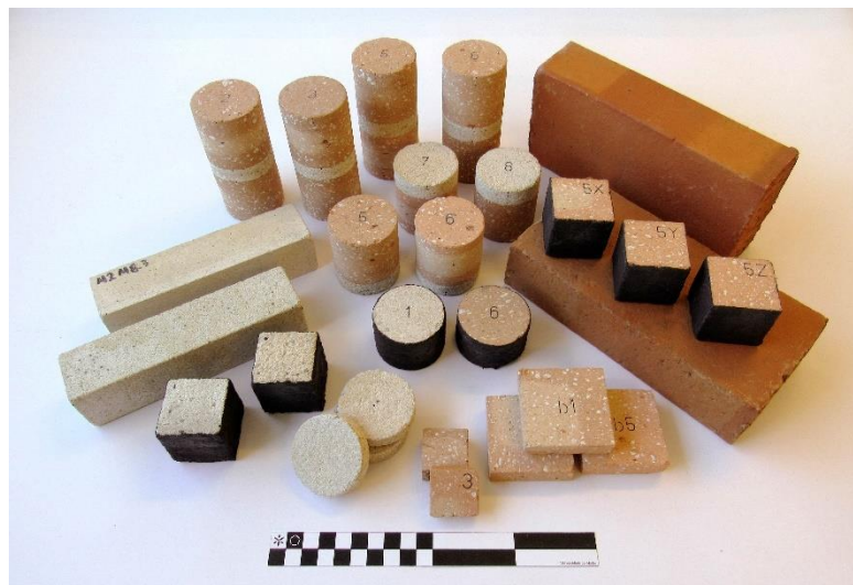
Figure 3.1. Selection of material samples: fired–clay brick, Portland cement mortar, natural hydraulic lime mortar (moulded and extracted from masonry bed joints), and masonry composites. The scale bar is 20 cm long.
