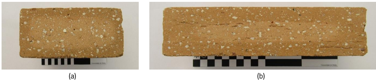
Figure 3.2. Cross-sections of fired-clay brick units: (a) transversal section through middle plane; (b) longitudinal section through middle plane.
