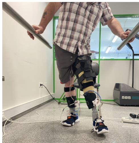
Figure 3-4: Devices worn by the participants in the research study. Vibrotactile Upper Leg Socket (VT-S) (I) and the subjects also wore on the feet Gait Shoes (II).
