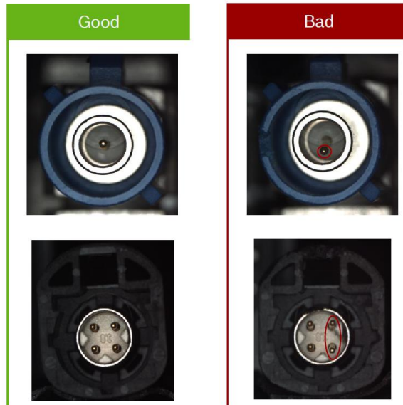
Figure 2 - Example of two different SC: Fakra (top) and HSD (bottom) and commonly associated defects.
