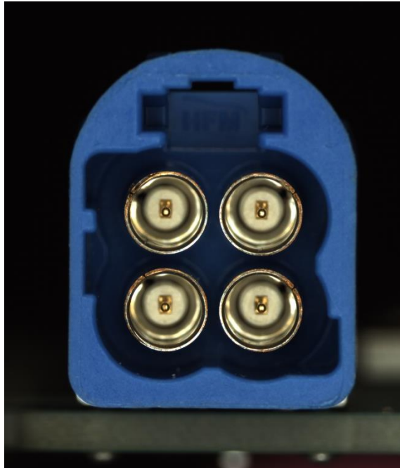
Figure 46 - Example of the small working range presented by Telecentric Optics. Though the pins are in focus, the back of the connector is not.
