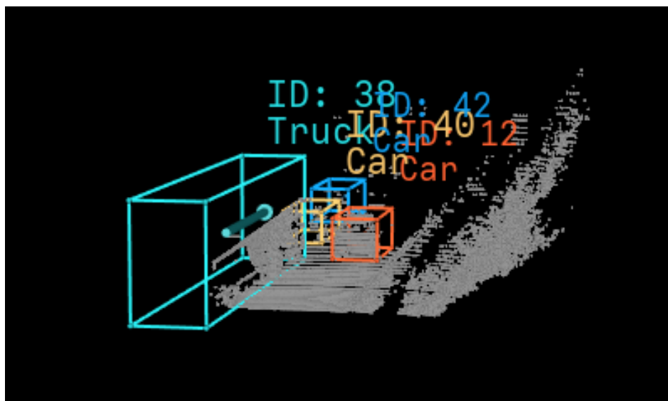
Figure 16: Example of KITTI dataset annotated 3D point cloud, obtained by [11]
