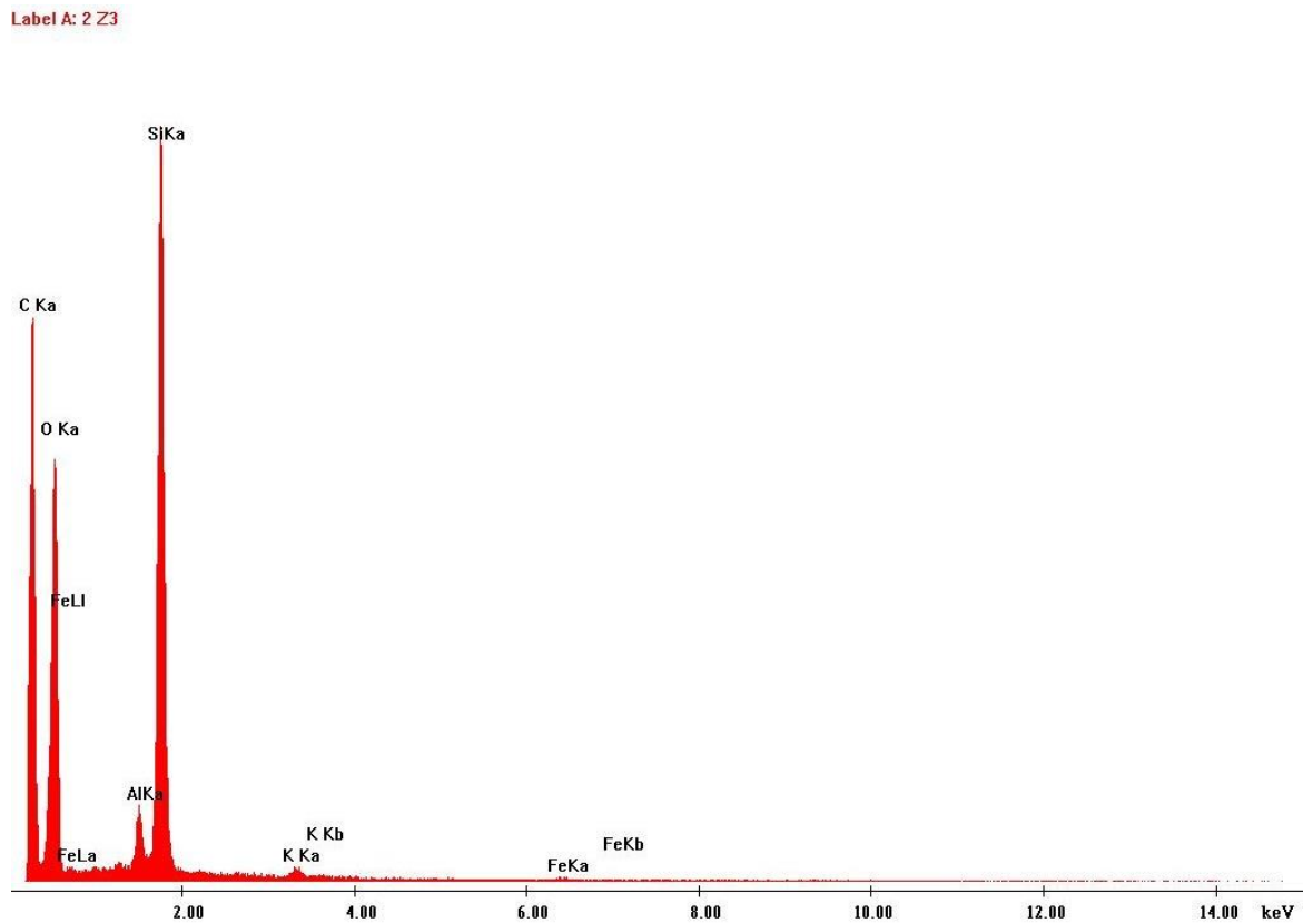
Figure 5.10. EDS analysis results: airborne sample collected on polycarbonate filter.
