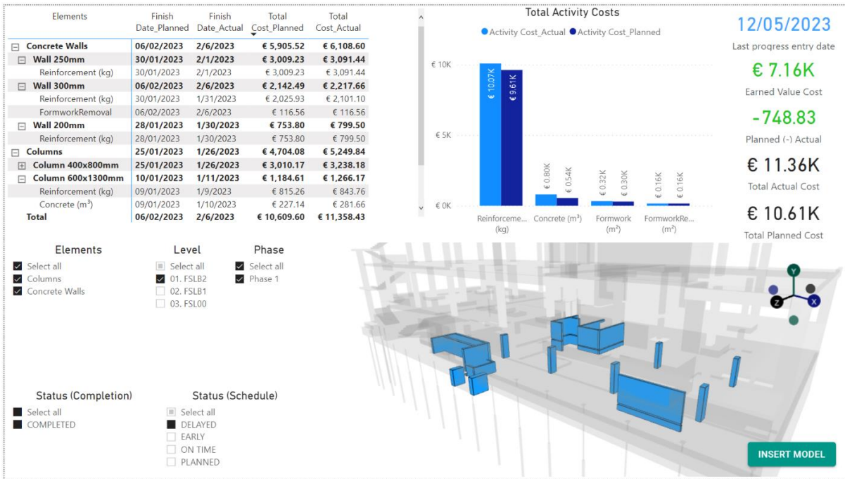
Figure 52. Template #1 for Progress Tracking, filtering the delayed elements on the first level
