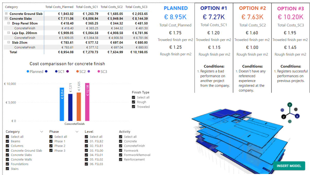
Figure 67. Template for E-Procurement filtered by the concrete finish activity
