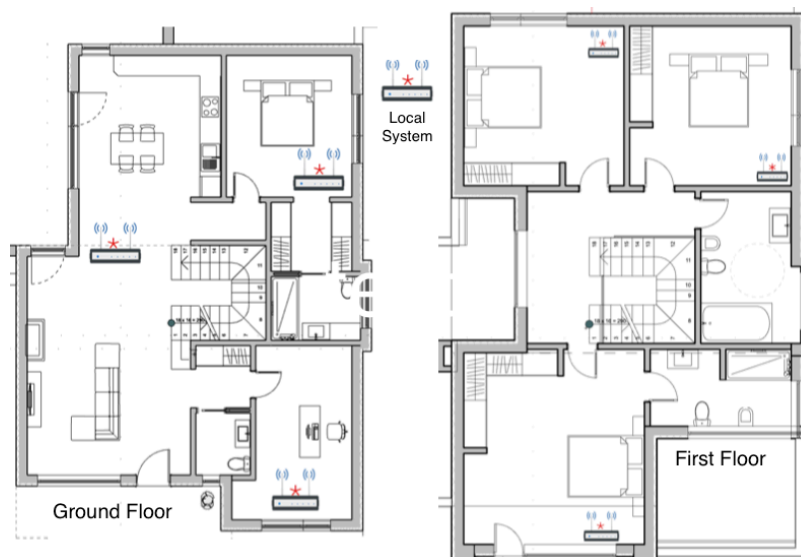
Figure 60: Home Scenario - Local System's installation.
