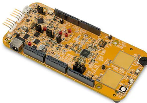
Figure 3.36: NXP S32K116 evaluation board
