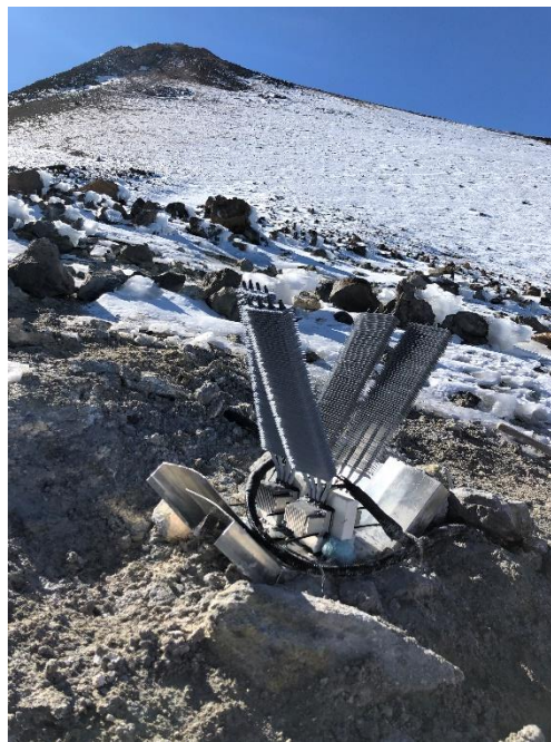
Fig. 1. Thermoelectric generator installed at Teide volcano in December 2019.
