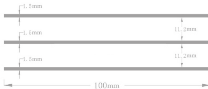
Figure 5 - Screen printing pattern used by Zhong et. al.
