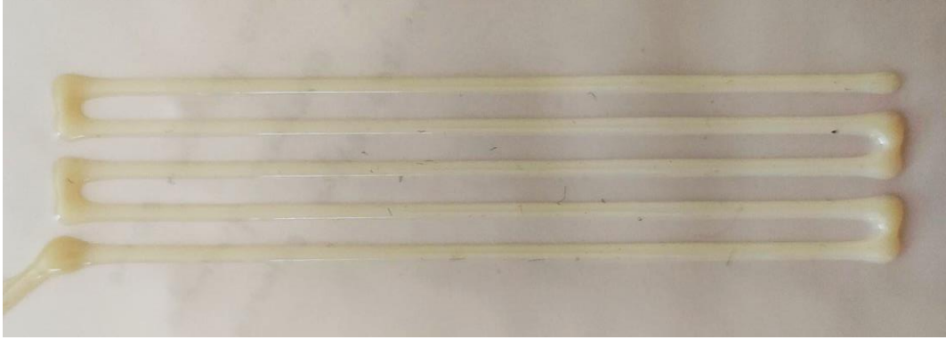
Figure 9 - Accumulation of silicon at the end of the printed lines
