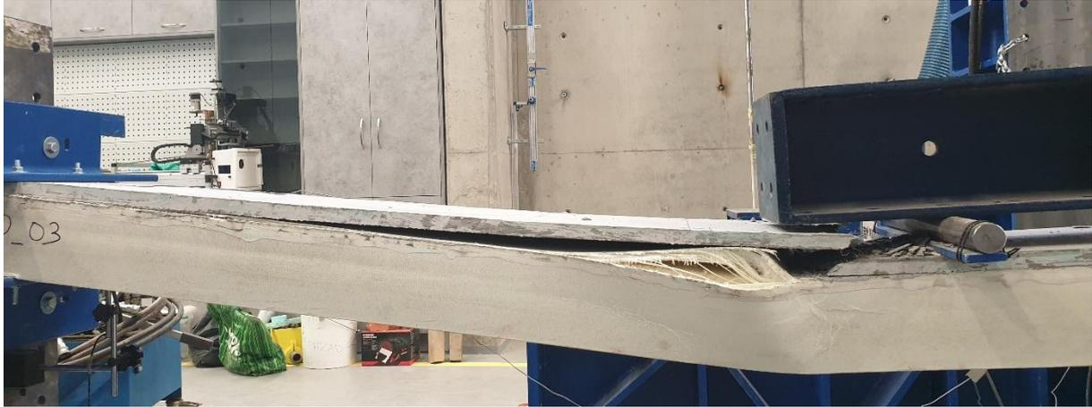
**Figura 94.** Modo de rotura do painel LT-2L\_1.
