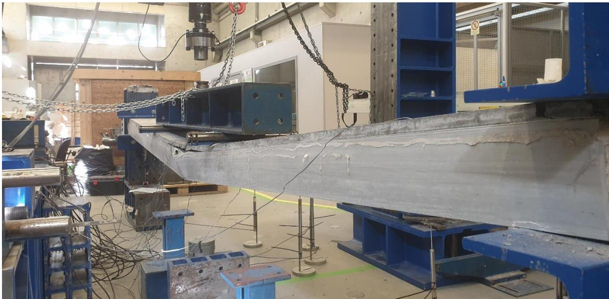
**Figura 95.** Modo de rotura do painel LT-2L\_2.
