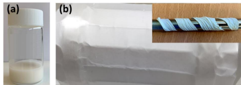
Figure 4. Perovskite polymeric solution (a) and MDABCO-NH 4 I 3 @PVC electrospun nanofiber mat (b) the inset shows a fiber mat folded around a cylindrical stick, demonstrating the flexibility of the fibers.
