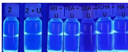
Figure A3 - Fluorimetric changes of BODIPY 2 with 50 equiv of each amine and U in ACN/phosphate buffer pH 6.5 (3:1), 2 hours after addition.
