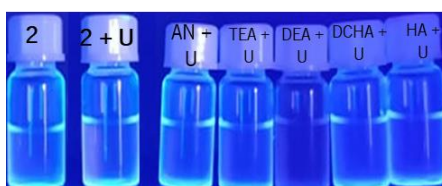
Figure 49- Fluorimetric changes of BODIPY 2 with 50 equiv of each amine and U in ACN/phosphate buffer pH 6.5 (3:1).
