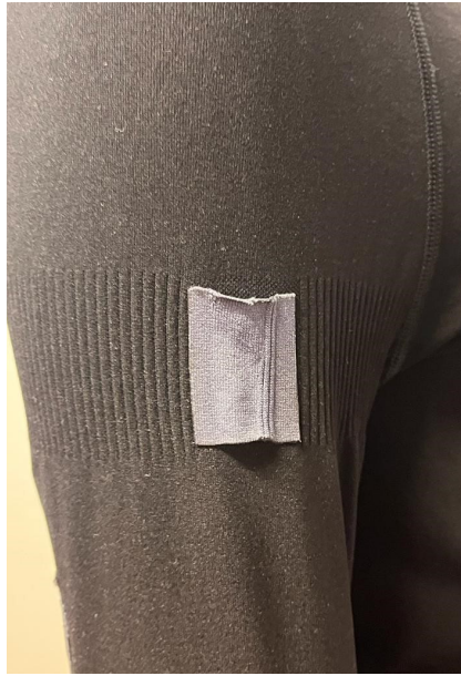
Figure 27: Vertical pattern mesh to help with the compression on the sensor area.
