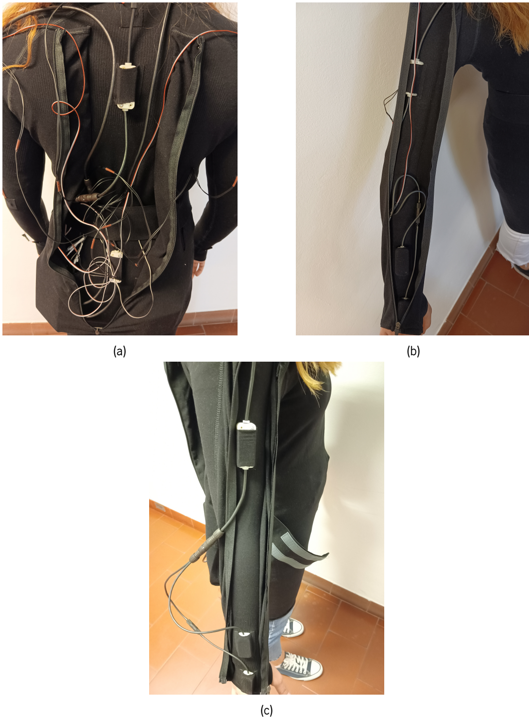
Figure 45: Overview of the wearable open. a) Rear view and b) side view. In c) the biofeedback system is absent, to showcase the connections between the modules.
