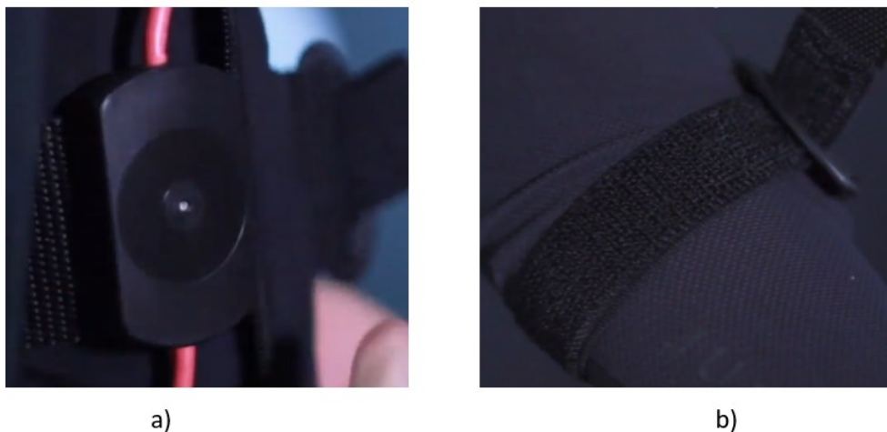
Figure 9: a) Attachments used in the Rokoko Smartsuit Pro, including b) tightening straps.
