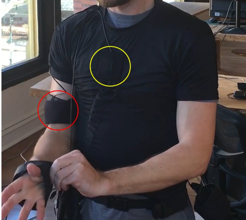
Figure 10: Attachments used in the shadow motion MoCap suit. Straps inside the red circle and pocket inside the yellow circle.
