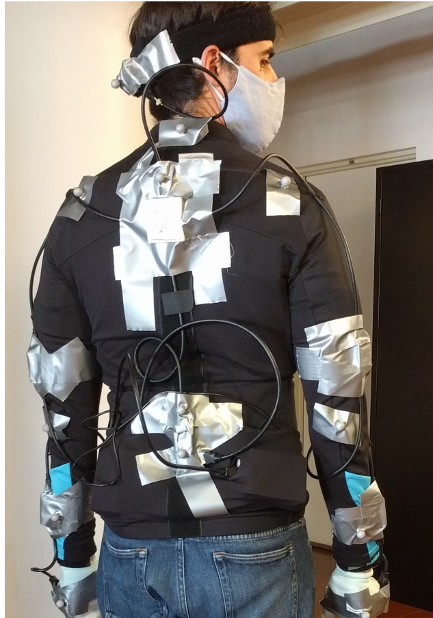
Figure 17: Adhesive tape used to fix the sensor modules onto the respective anatomical segment.
