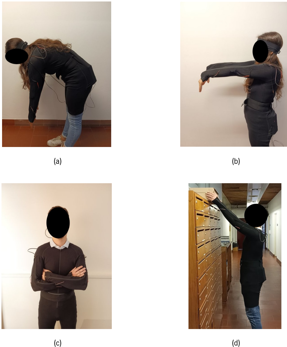
Figure 63: Movements performed by users during the ergonomic tests. a) Trunk flexion, b) wrist flexion, c) crossing arms and d) placing the box on top of the cabinet.
