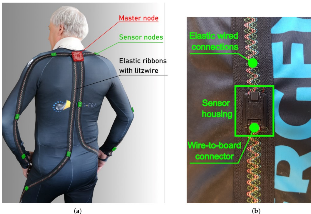
Figure 5: Proposed MoCap system. a) Overview of the setup. b) Zoom-in on the sensor module. Figure from [63].
