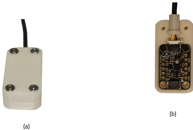
Figure 43: a) Extremity sensor module. b) Interior of the extremity sensor module.
