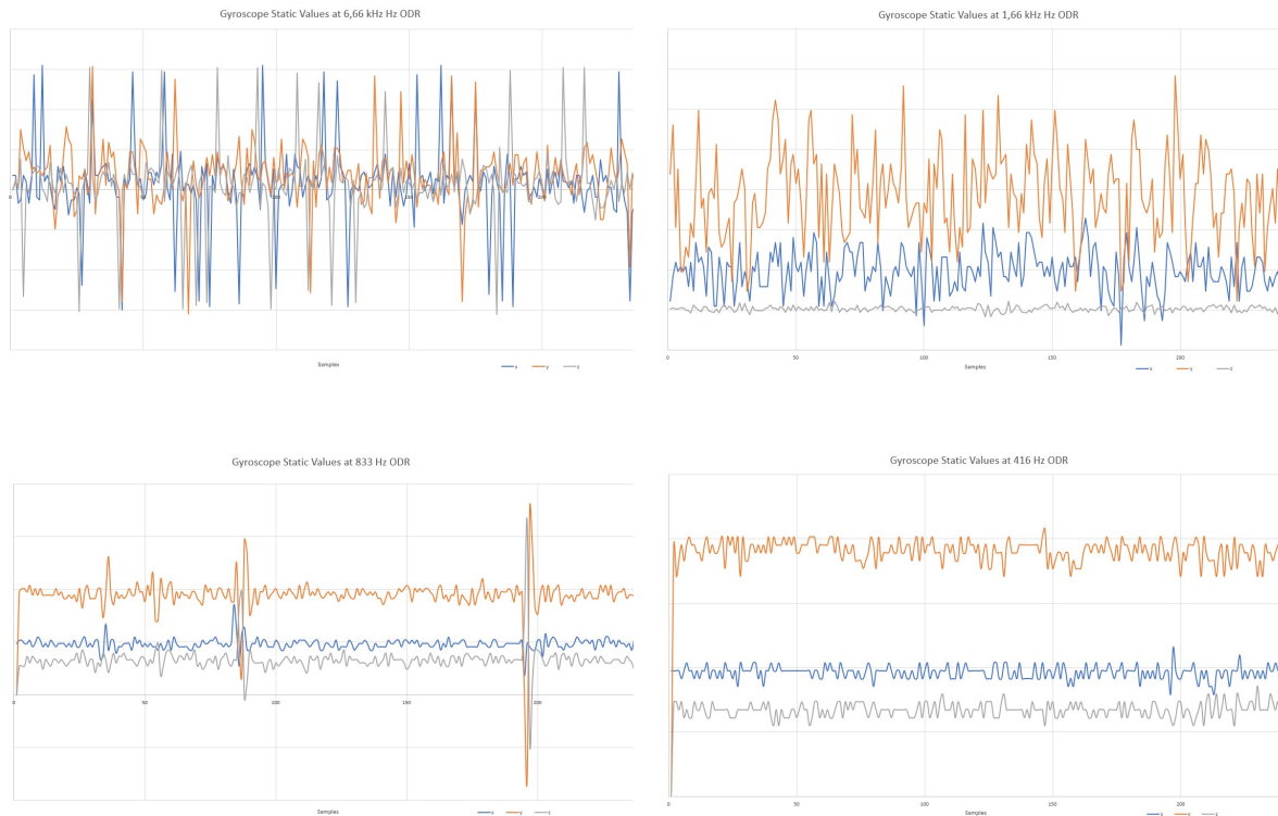
Figure 51: Angular velocity static outputs for different ODR configurations.
