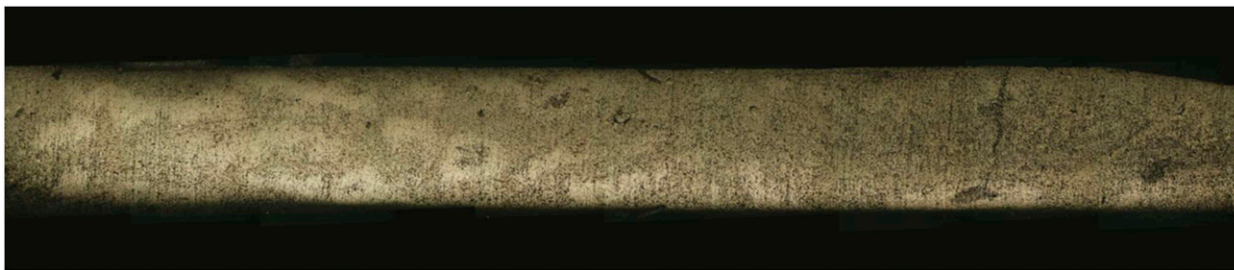
Figure 10. Cross-section analysis of laminate profile of CompTape.
