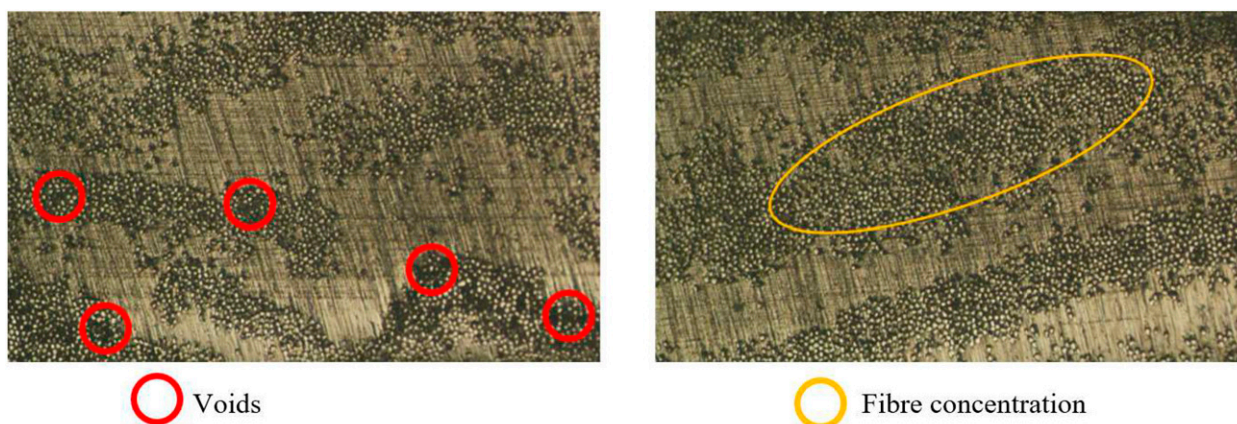
Figure 9. Close-up images of microscopy of pultruded profile (50x).
