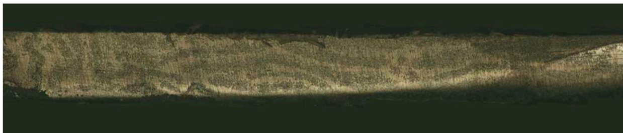
Figure 8. Cross-section of pultruded composite profile.
