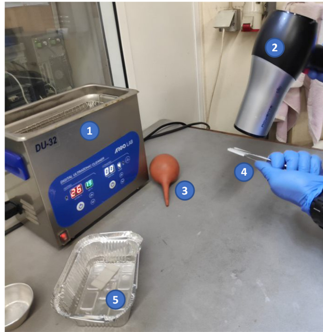
Figure 3.11. Equipment used in the density experiment: a DU-32 Argo Lab digital ultrasonic cleaner (1), a hair dryer (2), rubber ear wash ball (3), a set of tweezers (4), and an aluminium foil container with ethanol (5). Additionally, a Mettler AE240 precision analytical digital balance scale with a small structure to support the test specimens and a beaker with distilled water were used but are missing from this image.
