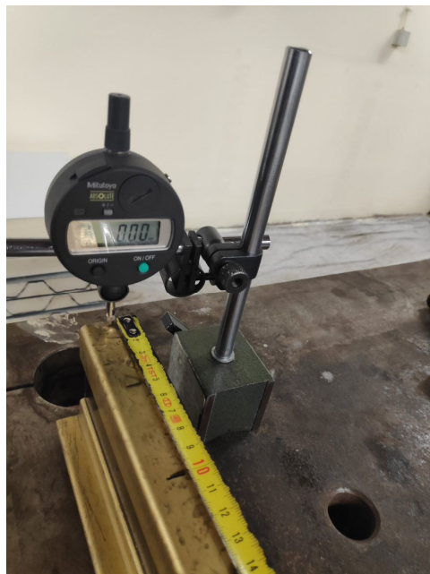
Figure 3.15. Digital gauge with a magnetic base on a steel table for the measurement of the residual deformation on the MMB, after the three-point bending experiment. Black lines can be seen every 50 mm that mark the measuring points, and the gauge is set to zero on the first measured extremity.
