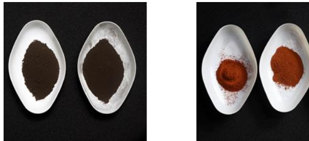
Figure 1: Left: Photograph of grey-colored titanium dioxide core ( \text{TiO}_2 ) and a copper oxide shell ( \text{CuO} ) powder pigment calcinated as 500^\circ\text{C} for 2h (left) and 4h (right); Right: Photograph of \text{Bi}_{1-x}\text{La}_x\text{FeO}_3 ( x=0.2 or 0.4 ) orange-colored pigments.
