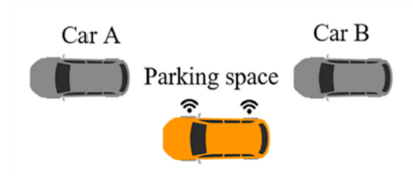
Figure 2.18: Schematic view of a parallel parking maneuver, where the ultrasonic sensors capture the parking space dimensions and relative position to the car. Figure from [4]. Author unreachable
