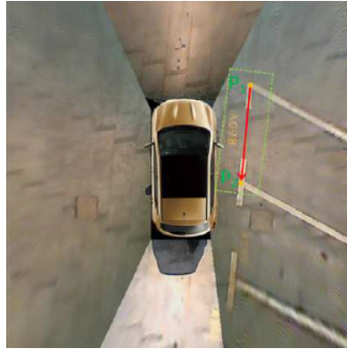
Figure 2.19: Parking spot detection using a AVM system. Figure from [5]. Author unreachable
