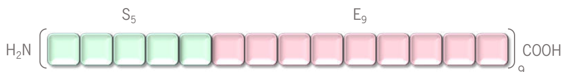
Figure 2. Representation of SELP-59-A construct. The polymer contains 9 repeats of a monomeric unit with 5 repeats of the silk consensus sequence GAGAGS (S 5 , green) and 9 repeats of the elastin-like sequence VPAVG (E 9 , pink).
