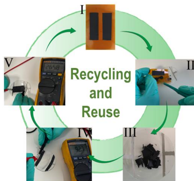
Figure 9- Recycling and reuse of the beeswax after screen-printing (I) over Kapton, then removed (II-III) and (IV-V) and heated at 60 °C for 10 min, showing low resistance values for pattern lines.
