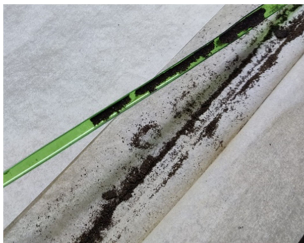
Image 9. Resulting product after the ironing, as we can see, the algae clearly didn't incorporate properly in the strip
