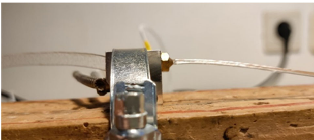
Image 10. Converting the PET strips into filament
