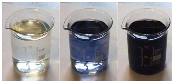
Figure 7. The solution color change after a period of time called the Landolt's time, When the iodine is reaches the maximum it forms a iodine-starch complex responsible of the dark-blue colour of the solution
