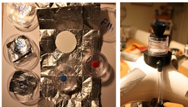
Figure 6. E-Drone Air inlet prototyping using filter filled sampling cassettes
