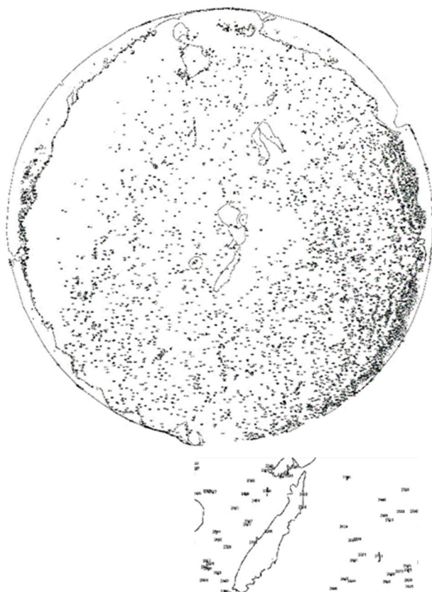
Figure 7. Microparticles counting in ImageJ of a Glass fiber filter with freshwater sediment and weathered polymers, stained with Nile Red and photographed under UV-light (particles=8 558; 62.517 pxmm -1 ; area range (mm 2 ))
