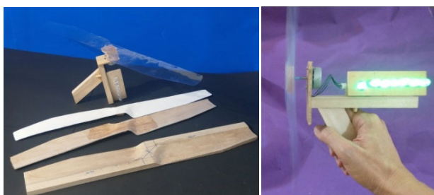
Figure 9. A finished wind turbine that can drive a tiny generator to light several LED (right). The mold used to form the shape of the wind turbine. The wind turbines made respectively of paper-based and balsa-wood-based composite materials, with a wind turbine made of PVC (left)
