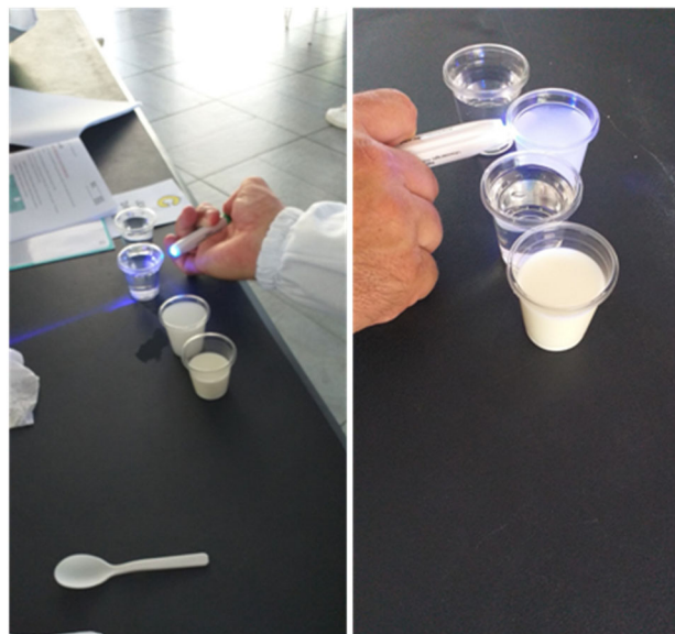
Figure 1. Tyndall effect in a sample of sucrose solution (left) and milk (right). The UV laser light is scattered only in the latter, which indicates the colloid nature of milk
