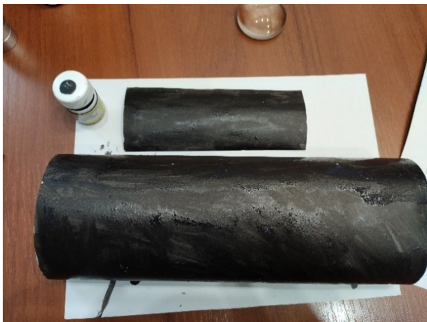
Figure 3. Black painting of the tube walls
