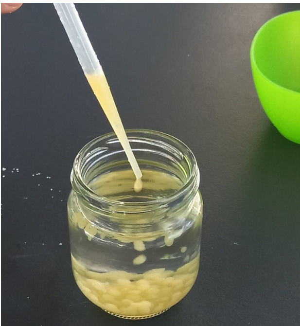
Figure 7. Direct spherification performed with a pasteur pipette
