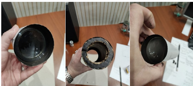
Figure 5. Creating a lens and eyepiece tubes
