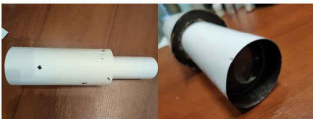
Figure 6. Simple refractor telescope in assembly
