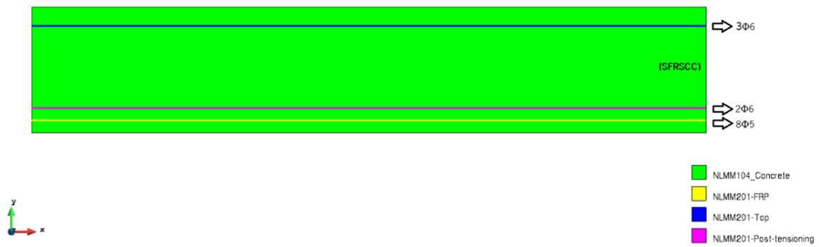
Figure 45 – GID graphic visualization of the assigned materials constitutive models in the B_8_45_Post Tensioning beam.
