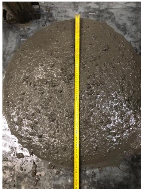
Figure 13 – SFRSCC slump flow test.
