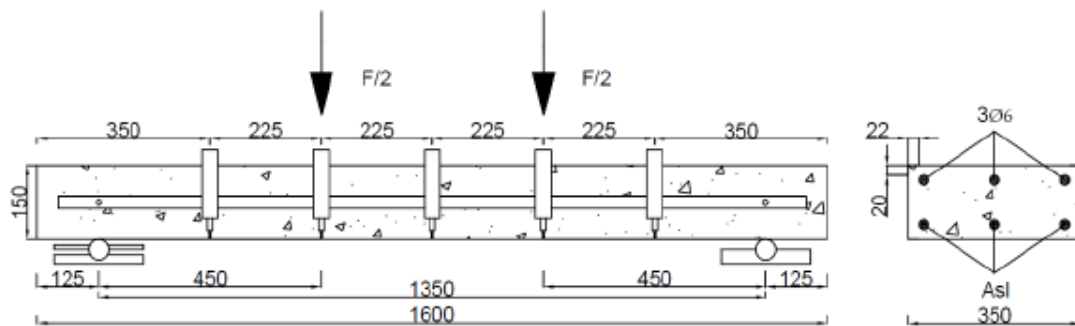
Figure 35 – Geometry, support and load conditions of the tested shallow beams including the monitoring system [35].
