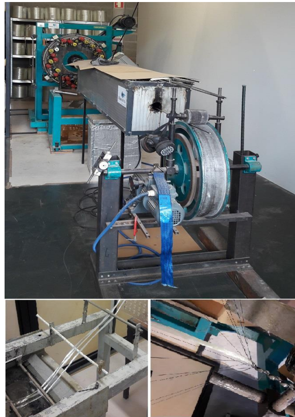
Figure 2 - Standard horizontal braiding machine developed by the Fibrous Materials Research Group, at University of Minho [17].
