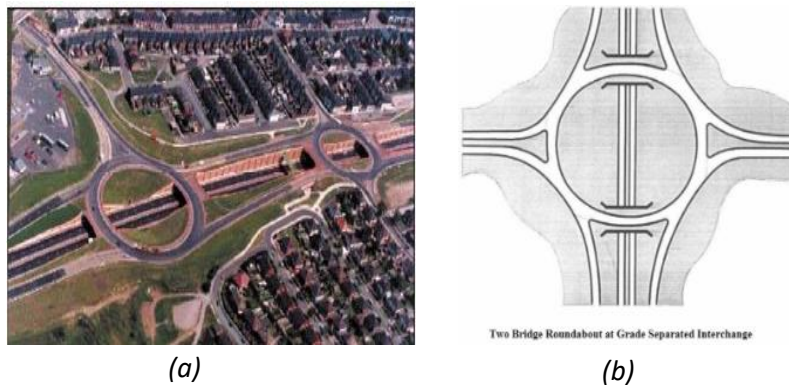
Figure 10 – (a) Example of Two Bridge Roundabout (FHWA, 2010)/ (b)- Layout of a Two Bridge Roundabout at Grade Separated Interchange (The Highway Agency, 1993).
