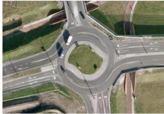
Figure 16 - Typical Turbo Roundabout in the Netherlands (Baranowski et al. , 2017)
