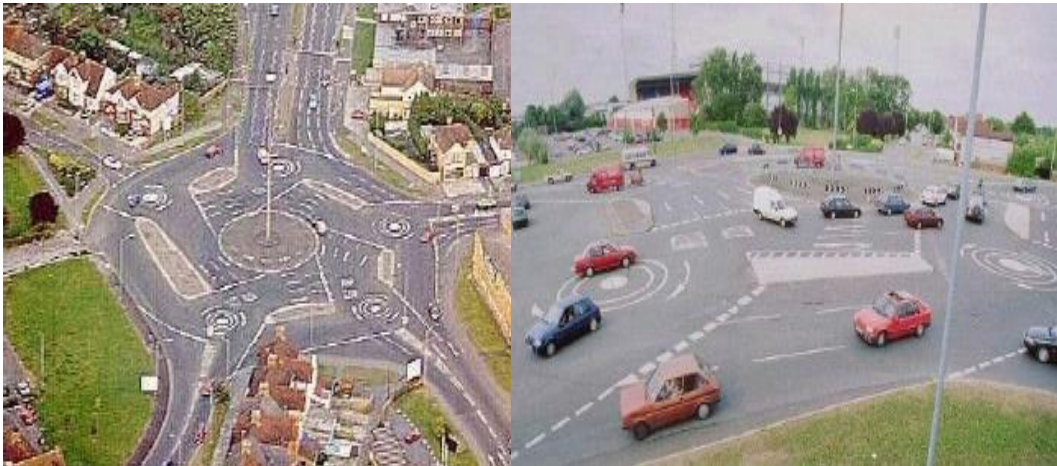
Figure 13 - Ring junctions (Kittelso, 2021)
