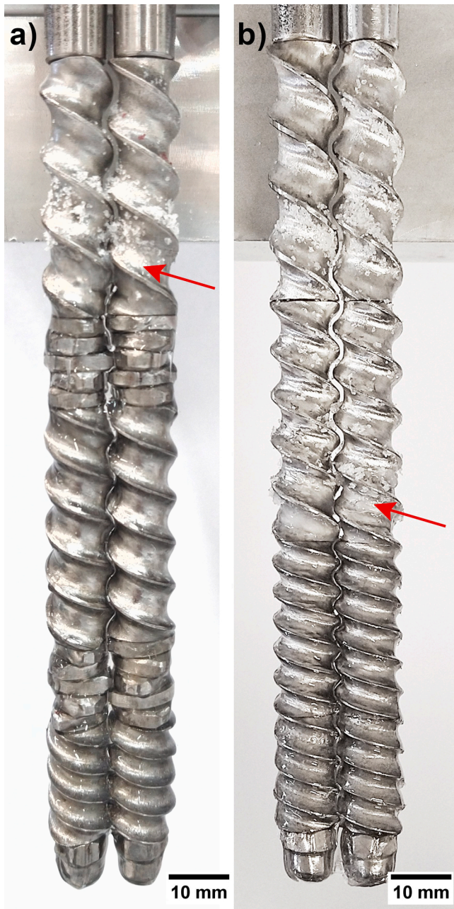
Fig. 8. Screw pull-out experiments evidencing the influence of the screw configuration on the melting location: (a) configuration 1; (b) configuration 2.
