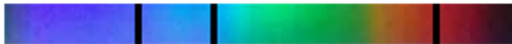
Figure 2. The spectrum of the Sun, taken with a spectroscope, shows the expected dark lines drawn by the students and considered to be the result of the existence of hydrogen.
