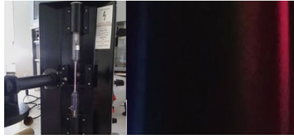
Figure 1. The light emitted from a lamp containing a heated gas of H_2 and its line spectrum.
