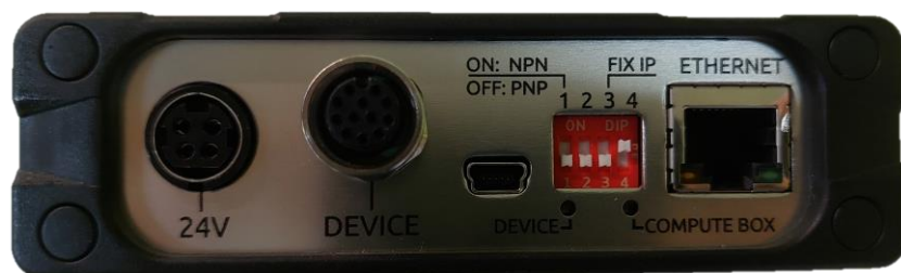
Figure 4.27 – Switches combination (in the gripper's compute box) that allows the attribution of a static IP.
