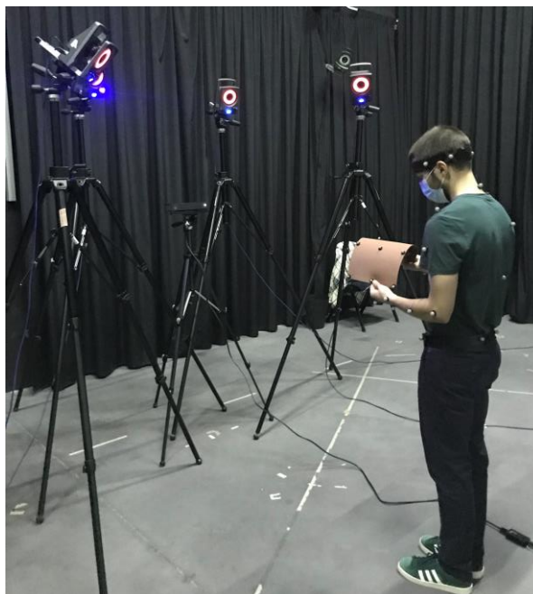
Figure 4.18 – 3D tracking system used in the orientations acquisition.
