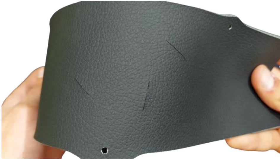
Figure 1.2 – Cut defects in a leather piece when it is bent.
