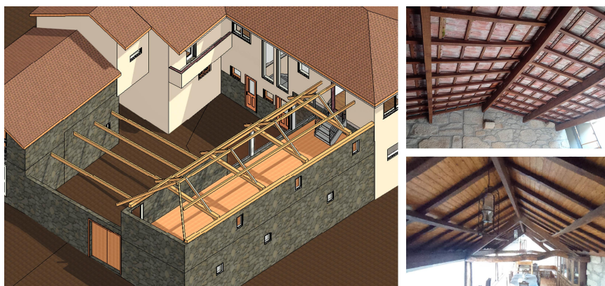
Figure 43 - Definition of roof structures' geometry
