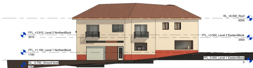
Figure 41 - Eastern facade with defined levels
