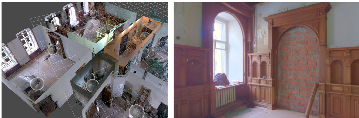
Figure 21 - Example of point cloud with panorama made by BLK360
