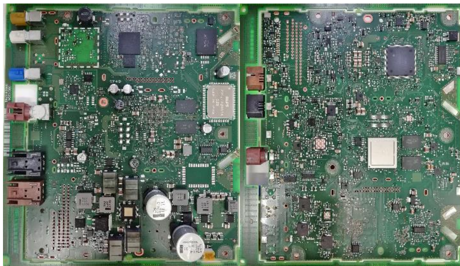
Figure 39 – Top (left) and bottom (right) side of the Renault IVI PCBA. This PCB had dimensions of 185 x 167 mm, an OSP surface finish and is one of the boards presently produced at BCM.
