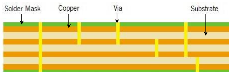
Figure 7 – Representation of a multilayer PCB [14] .
