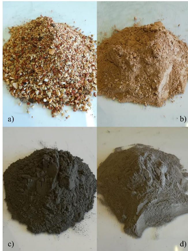
Figure 3-1. Precursors used in the laboratory experiments: a) original ceramic residue (CR); b) ceramic residue (MCR) milled for 32 hours, c) fly ash (FA), d) ladle furnace slag (LFS)
