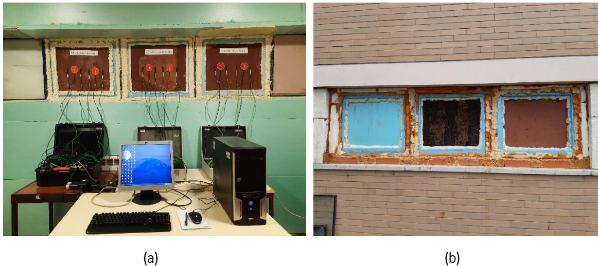
Figure 6-7. Thermal Experimental Setup of the half-sandwich panels, AAC + extruded polystyrene ( AP_{XPS} ), AAC + Insulation corkboard ( AP_{ICB} ), and the uninsulated panel (ACP): (a) sealed interior view; (b) sealed exterior view.
