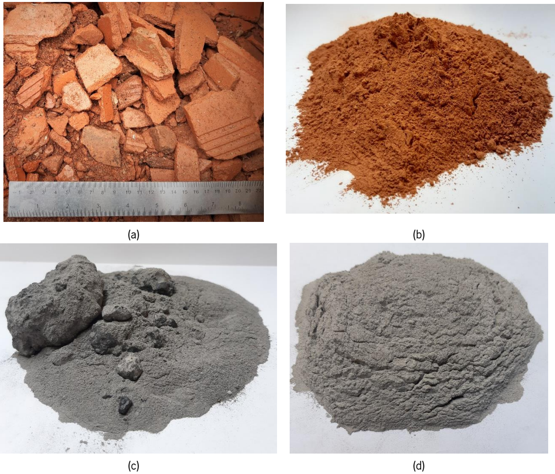
Figure 4-1. Precursors used in the mixture: (a) ceramic waste (CW) before grinding; (b) CW after grinding; (c) ladle furnace slag (LFS) before sieving; and (d) after sieving
