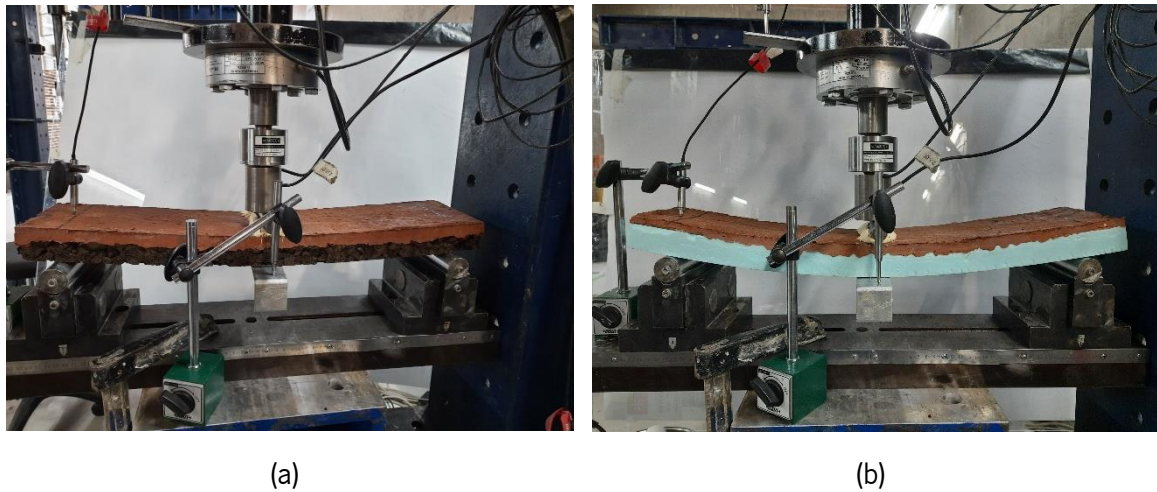
Figure 6-6. Set-up of the three-point bending test on half-sandwich AAC panels with different thermo-insulating materials: (a) extruded polystyrene (XPS) and (b) Insulation corkboard (ICB)
