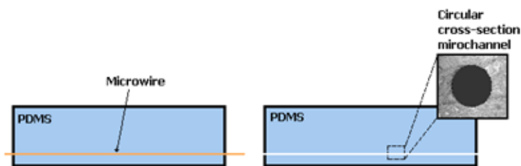
Figure 7. Schematic of the microwire-moulding methodology to fabricate PDMS circular cross-section microchannels. The microwire embedded in the PDMS (right side) is removed after the curing of the PDMS. As a result, it is possible to produce a circular microchannel (left side).
