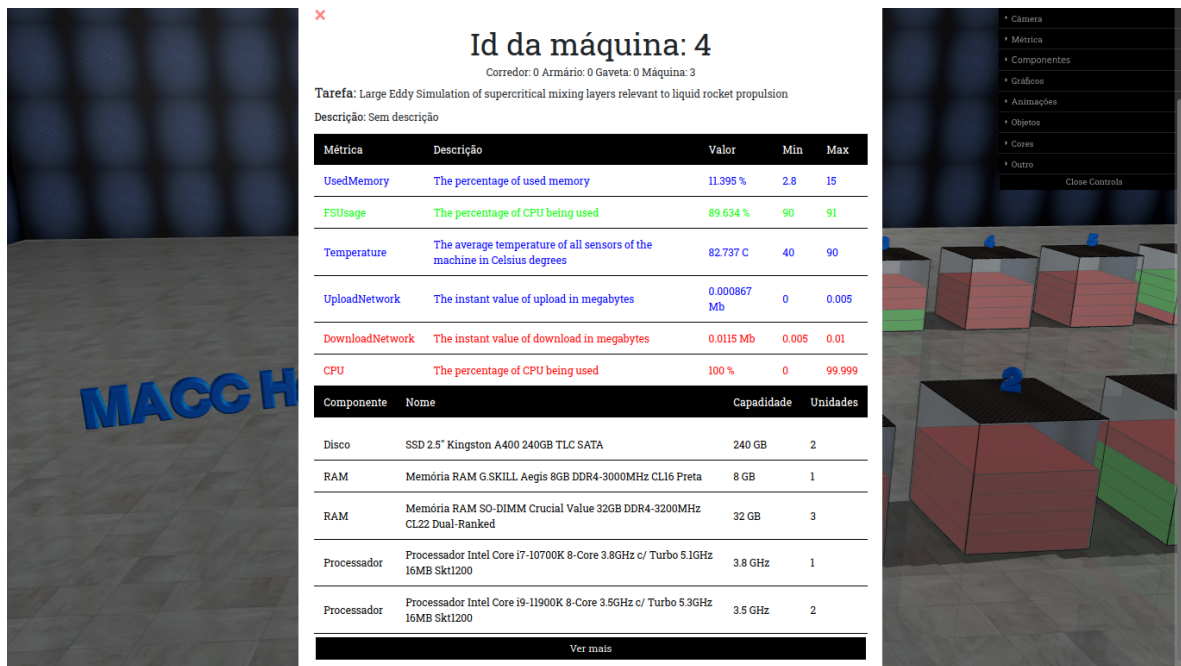
Figure 23: Popup with the performance, task, and components of a machine.
