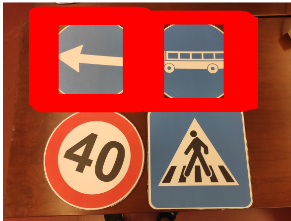
Figure 3.29: All the detections with confidence scores over 40%
