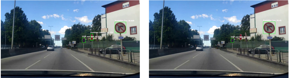
Figure 5.26: Detection of a sign not facing the camera from the YOLOV3 (left) and YOLOV3_tiny (right)
