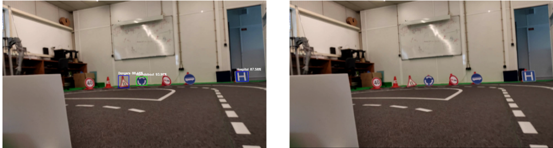
Figure 5.23: Detection with extreme distortion from the YOLOV3 (left) and YOLOV3_tiny (right)
