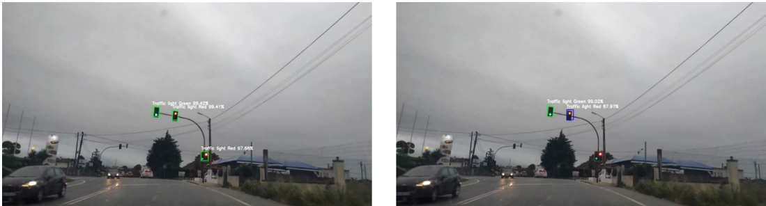
Figure 5.27: Traffic Light detection from the YOLOV3 (left) and YOLOV3_tiny (right)
