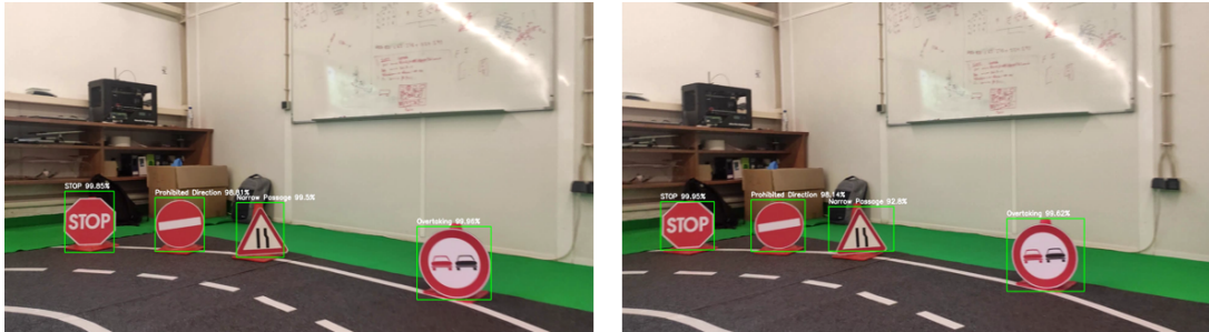
Figure 5.21: Bounding Boxes from the YOLOV3 (left) and YOLOV3_tiny (right)
