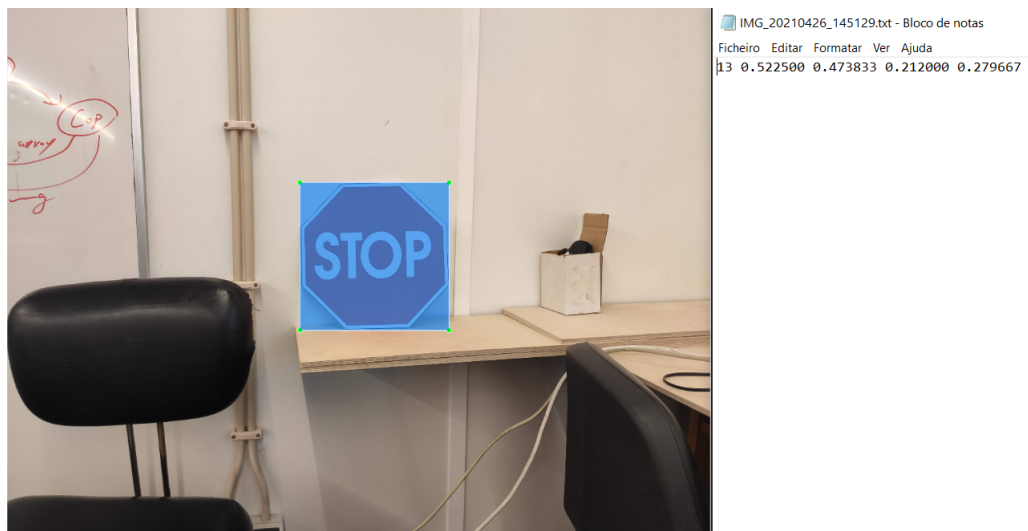
Figure 3.2: Image from one of the Datasets and its correspondent text file with the bounding box coordinates, dimensions and label
