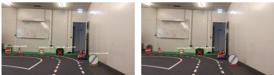
Figure 5.20: Detection distance from the YOLOV3 (left) and YOLOV3_tiny (right)
