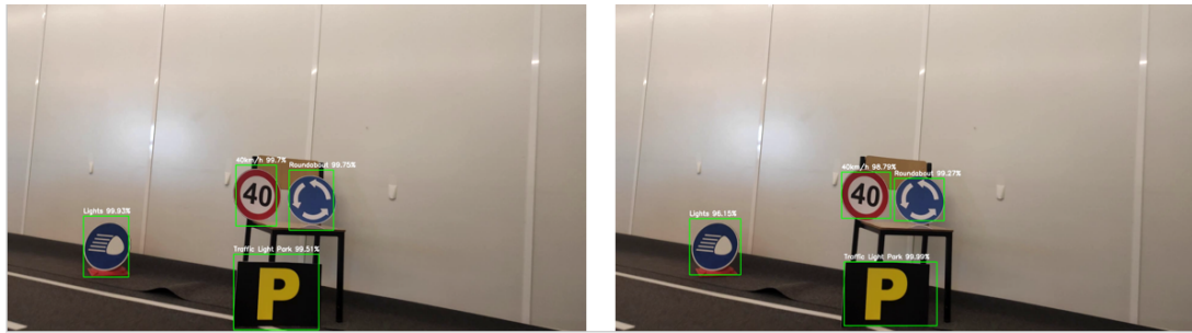
Figure 5.19: Detection from the YOLOV3 (left) and YOLOV3_tiny (right)
