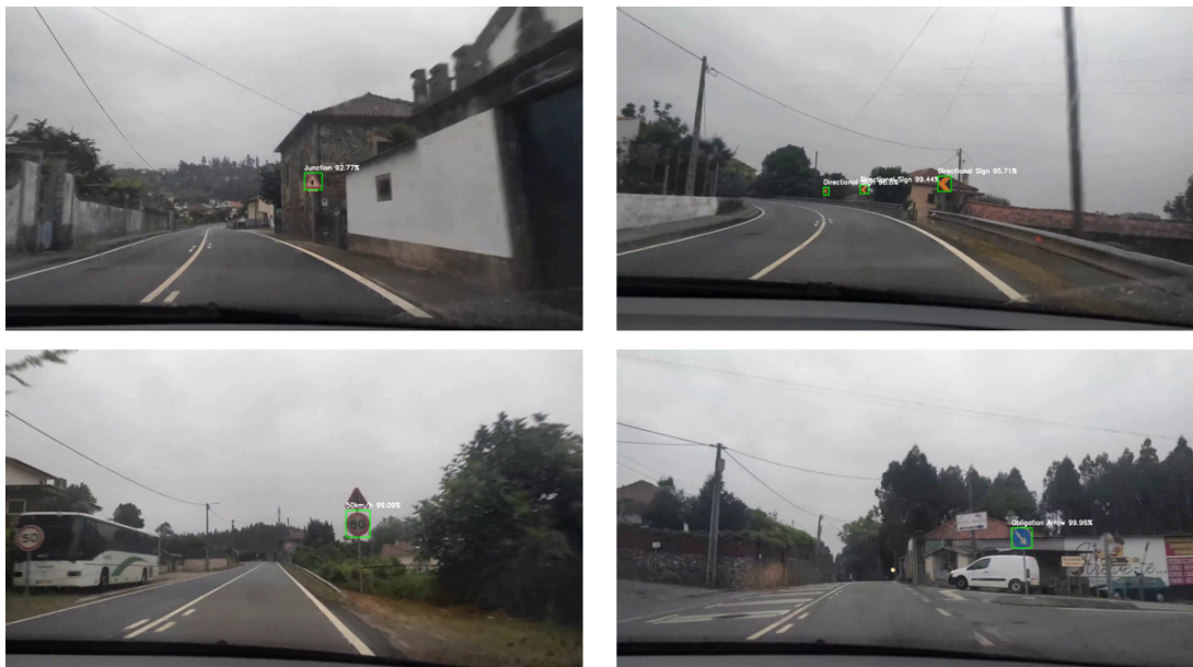
Figure 5.29: Results of the YOLOV3 network in poor conditions
