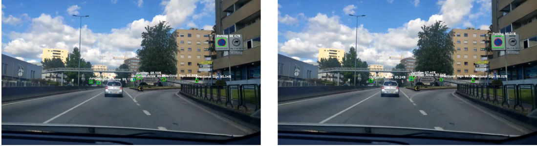
Figure 5.24: Detection with ideal conditions from the YOLOV3 (left) and YOLOV3_tiny (right)
