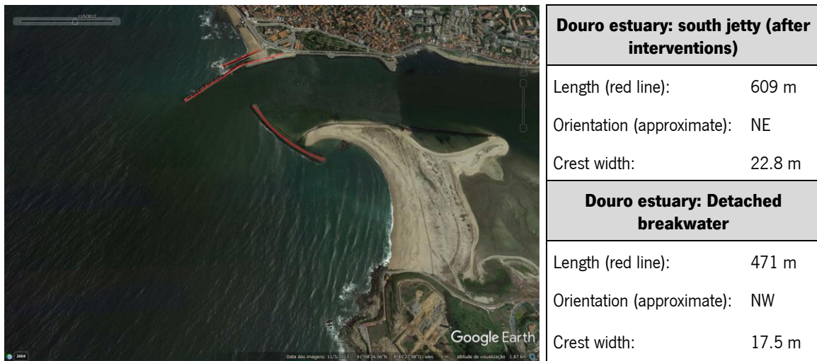
Figure 5.4: Douro estuary: characteristics after south jetty extension and detached breakwater construction (2013).
