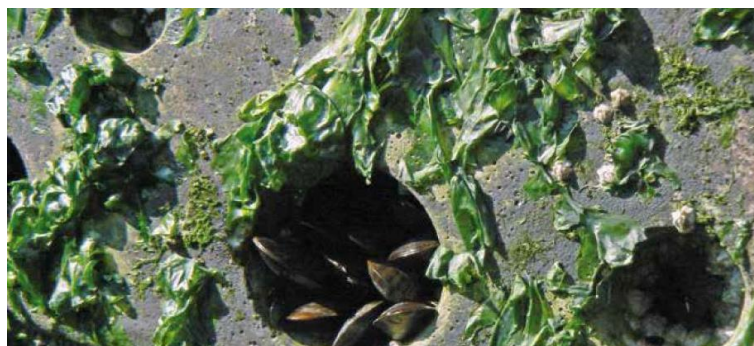
Figure 2.42: Eco concrete (Deltares, 2013).
