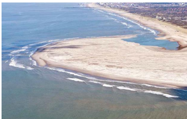
Figure 2.36: Sand engine (Deltares, 2013).
