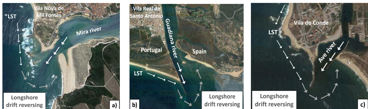
Figure 2.11: Longshore drift reversing: a) in Mira river estuary, Portugal (2015); b) at a jetty in Guadiana river estuary, southern Portugal and Spain border (2017); and c) at the jetties in Ave river estuary, Portugal (2017).
