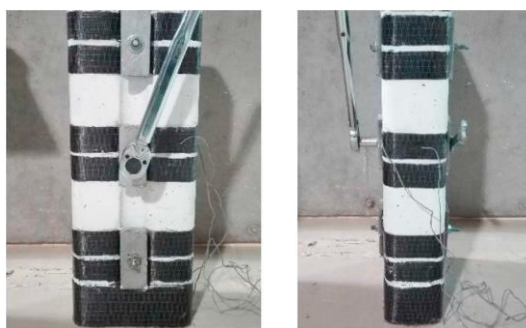
Figure 2.50: Representation of the prestress application on the FRP strips (Janwaen et al. , 2019).
