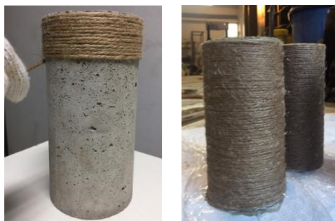
Figure 2.51: Wrapping process of dry rope to the concrete specimen (Suparp et al. , 2017).
