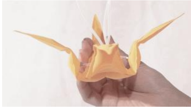
Figure 2.17. aeroMorph: a crane origami using pneumatic actuation. Republished with permission of ACM (Association for Computing Machinery), from Proceedings of the 29th Annual Symposium on User Interface Software and Technology , (Ou et al., 2016), copyright © 2016 ACM; permission conveyed through Copyright Clearance Center, Inc.
