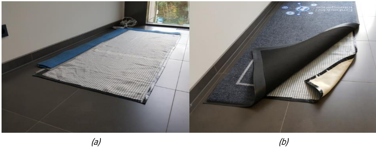
Figure 5.2. Piezoresistive sensing carpet: (a) fabric-based sensor and (b) operating under a real carpet. Reprinted from (Zhou et al., 2017), copyright © 2017, IEEE.
