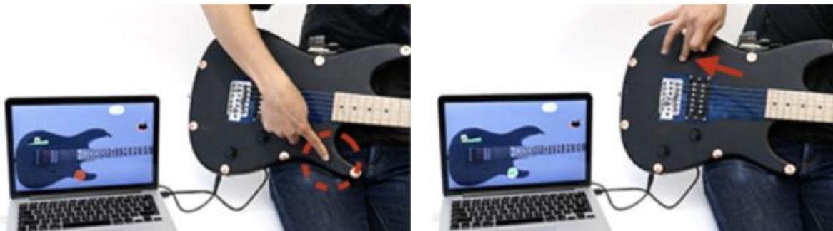
Figure 2.6. Electrick: a low-cost technique to assess touch input on objects or surfaces, even in non-flat ones. Illustration shows a guitar that was sprayed with carbonaceous ink to create touch buttons and sliders. Republished with permission of ACM (Association for Computing Machinery), from Proceedings of the 2017 CHI Conference on Human Factors in Computing Systems , (Yang Zhang et al., 2017), copyright © 2017 ACM; permission conveyed through Copyright Clearance Center, Inc.
