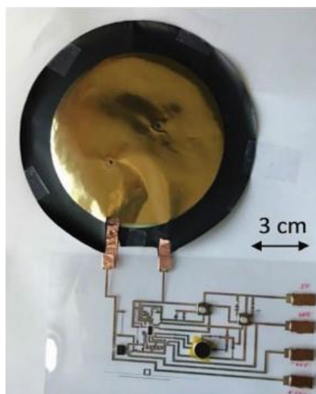
Figure 4.26. Bimorph P(VDF-TrFE) speaker with flexible and printed electronics.
