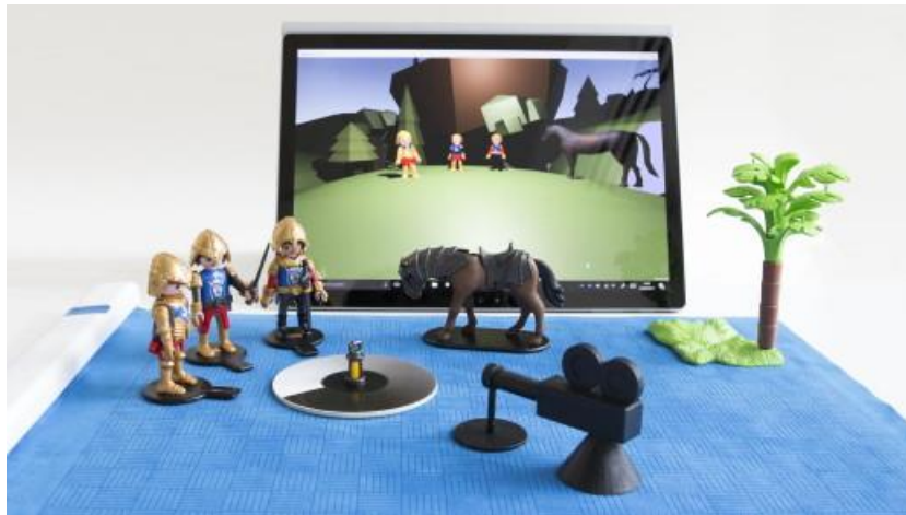
Figure 2.11. Project Zanzibar: a flexible mat capable of detecting objects placed on it via NFC, and their location via capacitive sensing. Republished with permission of ACM (Association for Computing Machinery), from Proceedings of the 2018 CHI Conference on Human Factors in Computing Systems , (Villar et al., 2018), copyright © 2018 ACM; permission conveyed through Copyright Clearance Center, Inc.
