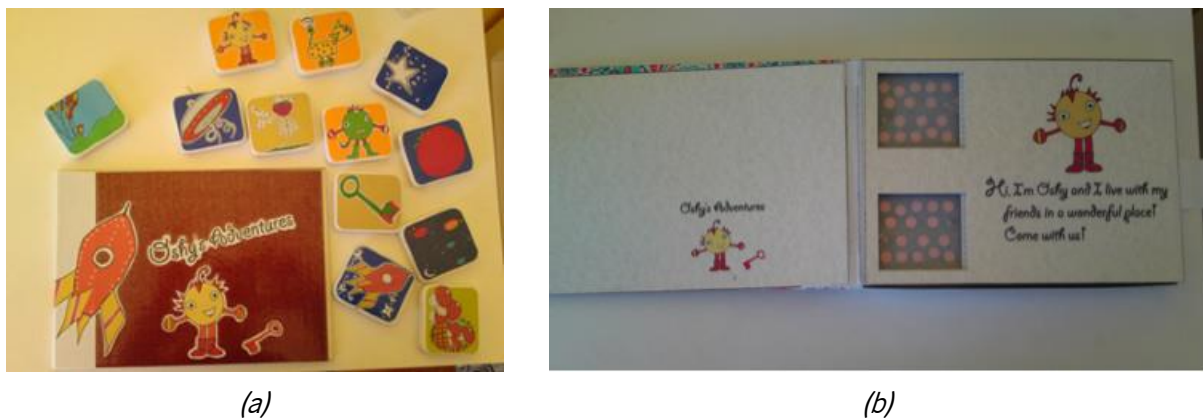
Figure 3.14. t-books prototype, (a) an adventure book with cards that are (b) placed in slots and detected through capacitive sensing. Republished with permission of ACM (Association for Computing Machinery), from Proceedings of the 11th International Conference on Interaction Design and Children , (Sylla, Gonçalves, Branco, et al., 2012), copyright © 2012 Authors.
