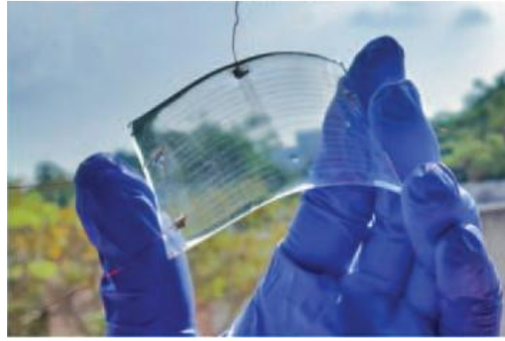
Figure 3.18. Transparent and flexible interdigitated capacitive sensor. Republished with permission of IOP Publishing, Ltd., from Flexible and Printed Electronics , (Nair et al., 2019), vol. 4(4), copyright © 2019 IOP Publishing Ltd.; permission conveyed through Copyright Clearance Center, Inc.
