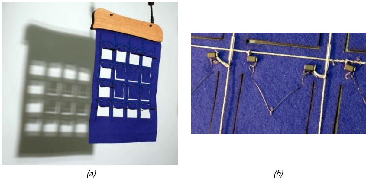
Figure 2.14. Shutters: (a) kinetic shadow window display and (b) detail of the levered windows using SMAs. Republished with permission of ACM (Association for Computing Machinery), from Proceedings of the 3rd International Conference on Tangible and Embedded Interaction , (Coelho & Maes, 2009), copyright © 2009 ACM; permission conveyed through Copyright Clearance Center, Inc.
