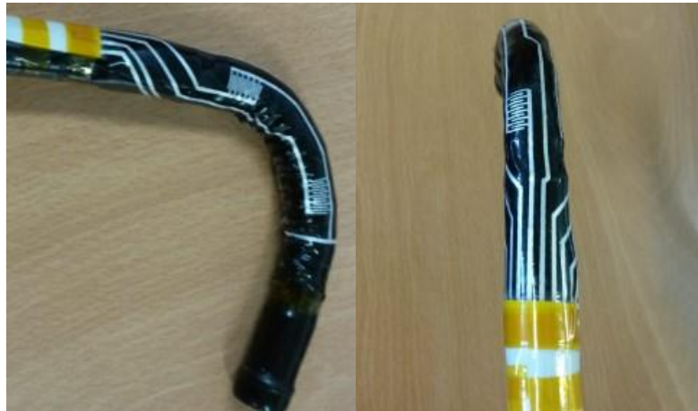
Figure 2.19. Example of the versatility of polymer films: Sensor matrix wrapped around an endoscope.
