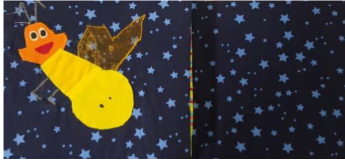
Figure 2.10. Hello World book prototype, a textile touch-and-feel book with embedded electronics (two dots in the firefly are a light sensor, and stars are LEDs).
