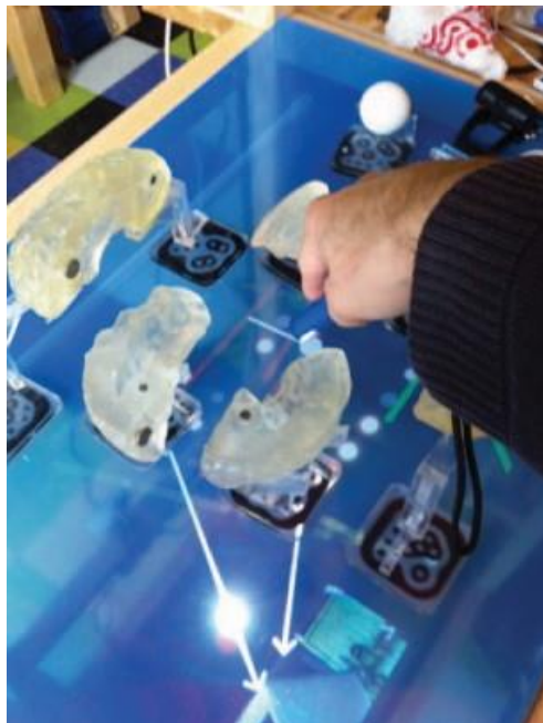
Figure 2.7. BrainExplorer, a TUI for neuroscience teaching and learning. Reprinted from (Schneider et al., 2013), copyright © 2013, IEEE.
