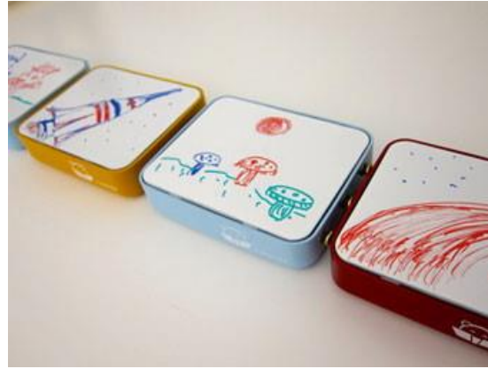
Figure 2.12. t-words: a set of audio record and playback blocks for language exploitation. Reprinted by permission from Springer Nature, Creativity in the Digital Age , (Sylla et al., 2015), copyright © 2015, Springer-Verlag London.
