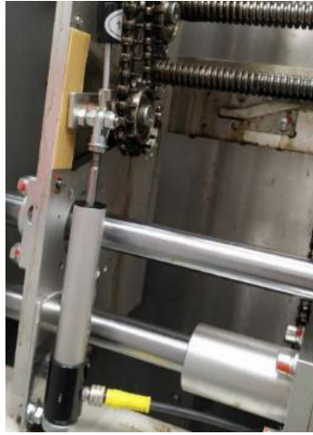
Figura 59 – Potenciômetro linear “Novotechnik TX2 0050-716-002-101”.
