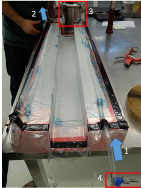
Figure 5.15 - Infusion vacuum setup to switch on the vacuum
