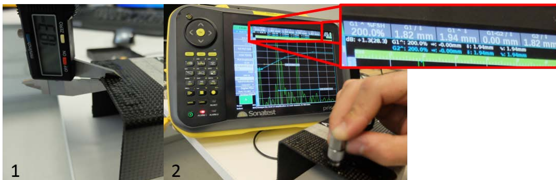
Figure 5.22 - Measuring the thickness of external shell composite part: 1) with a calliper; 2) with the ultrasound probe
