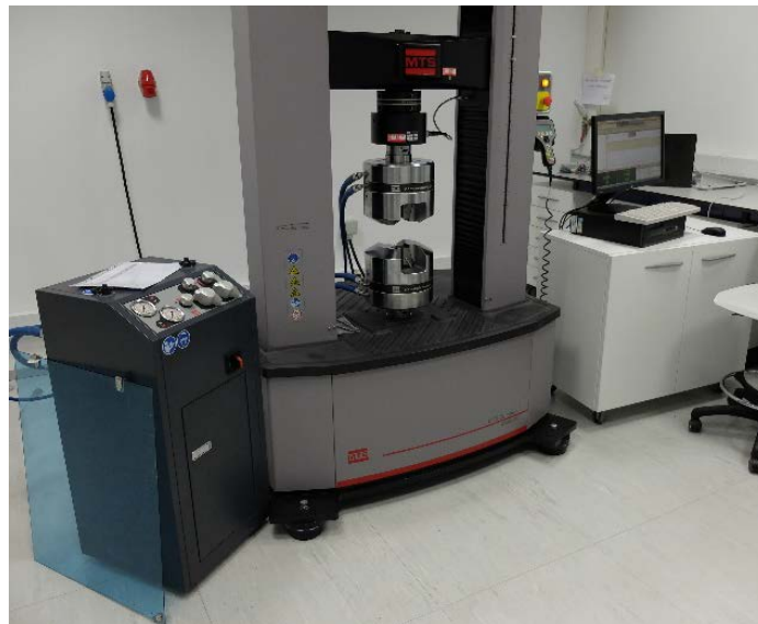
Figure 5.4 - Universal testing equipment used for mechanical testing
