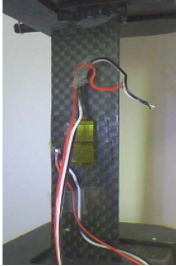
Figure 6.22 - Sample presenting the most common type of failure observed (code LAT of ASTM aD3039/D3039M-08)
