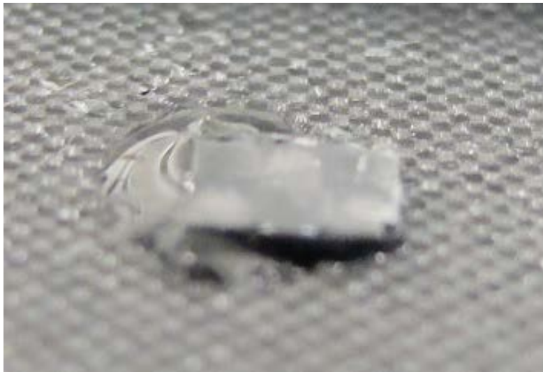
Figure 5.19 - Small laminate squares used to control the adhesive layer thickness
