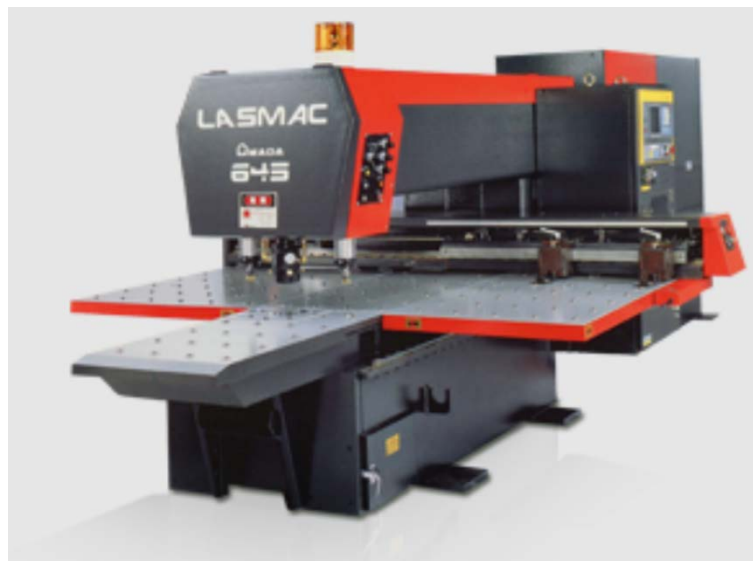
Figure 2.1 – Fixed optics ILCM Amada Lasmac 645 [13]
