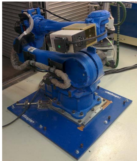
Figure 5.7 - Robotic set used for machining the polyurethane based moulds.
