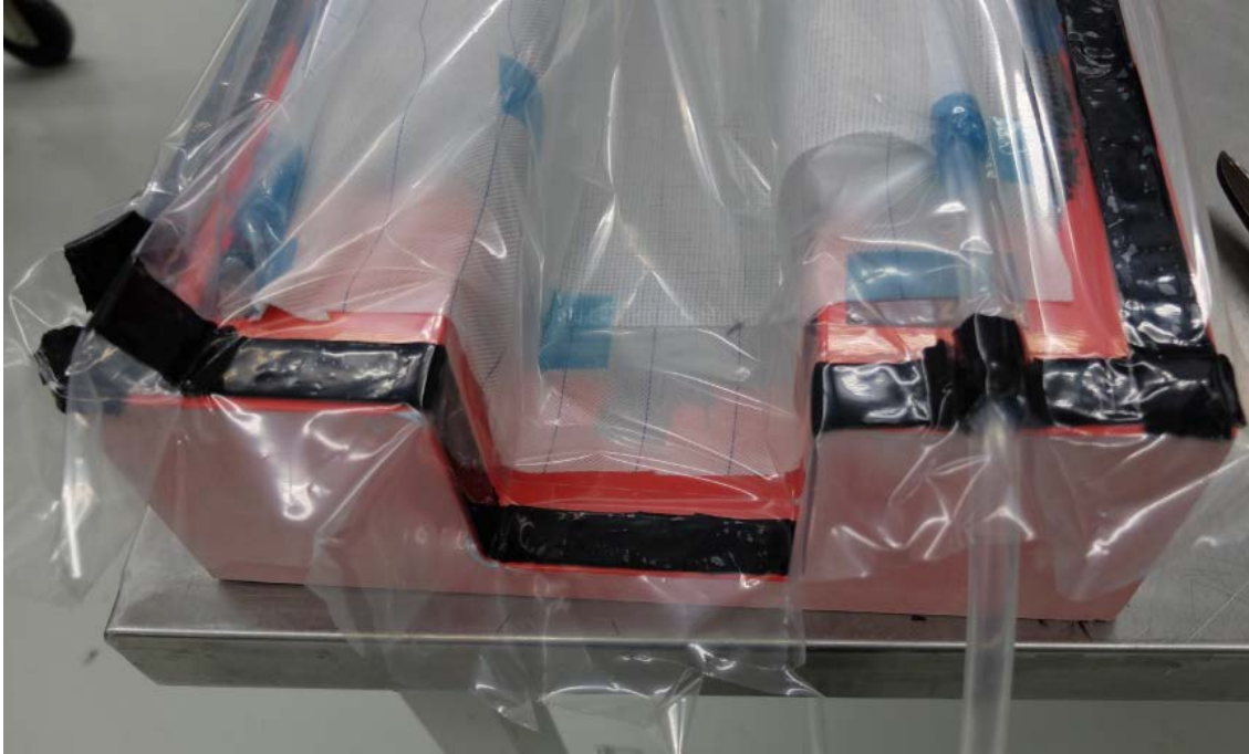
Figure 5.14 - Final setup of the vacuum infusion mould
