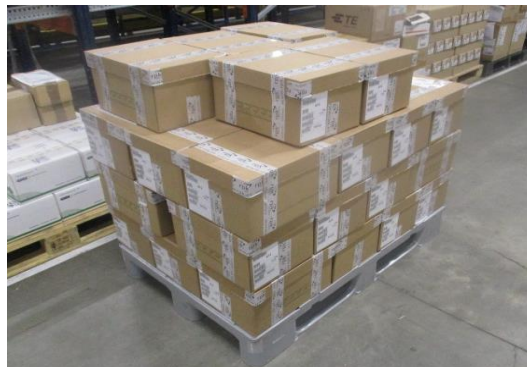
Figure 61. Material stored on non-standard pallets
