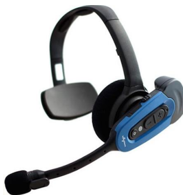
Figure 23. Example of AAR system: Vocollect (Reproduced from: ILS (2017))
