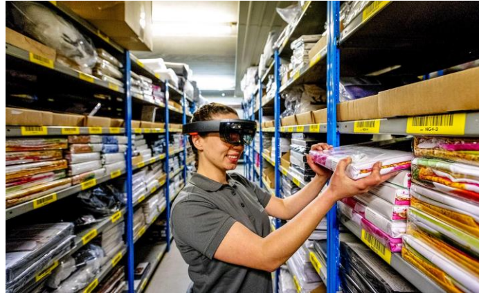
Figure 25. Operator using a HMD to support order picking process (Reproduced from: Marsh McLennan (2021))
