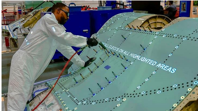
Figure 22. Example of SAR: Projected work instructions on F-35 aircraft assembly line (Reproduced from: Aerospace Manufacturing & Design (2015))
