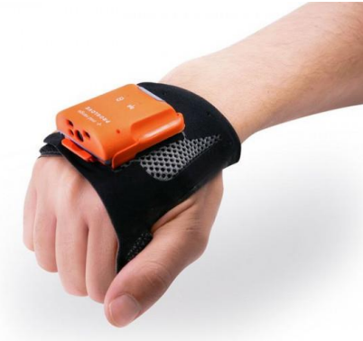
Figure 21. Example of WWD: Proglove Mark 2 (Reproduced from: Etiden (2020))
