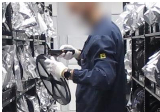
Figure 59. Operator scanning a reel's barcode with PDA
