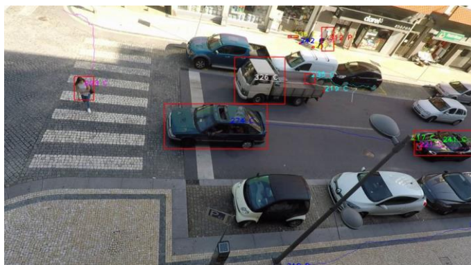
Figure 2.4 – Example of the video analysis made through Traffic Intelligence (BMJ street, Braga).
