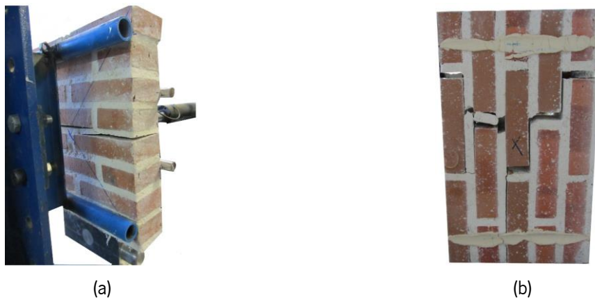
Fig. 6-4. Failure mode of unreinforced flexural panels: (a) UP; (b) UN.
