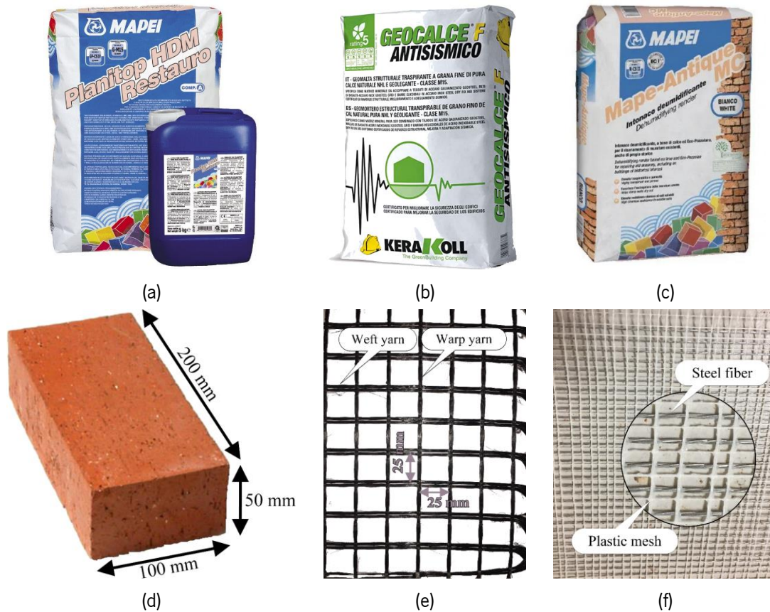
Fig. 3-1. Materials used: (a) mortar M1; (b) mortar M2; (c) mortar M3; (d) clay brick; (e) glass fabric; (f) steel fiber.
