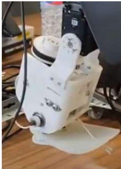
Figure 3.38 - DARwIn prosthetic attached with revised attachment method
