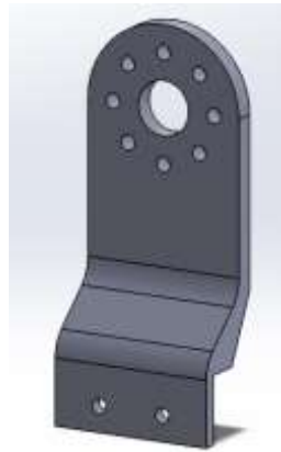
Figure 3.37 - Second iteration of the prosthesis-knee attachment component
