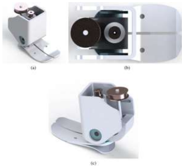
Figure 3.8 - CAD model of the DARwIn-OP prosthesis with a) isometric, b) top and c) rear views [1]
