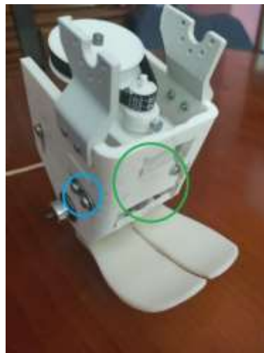
Figure 3.24 - Prosthesis fit with modified main body
