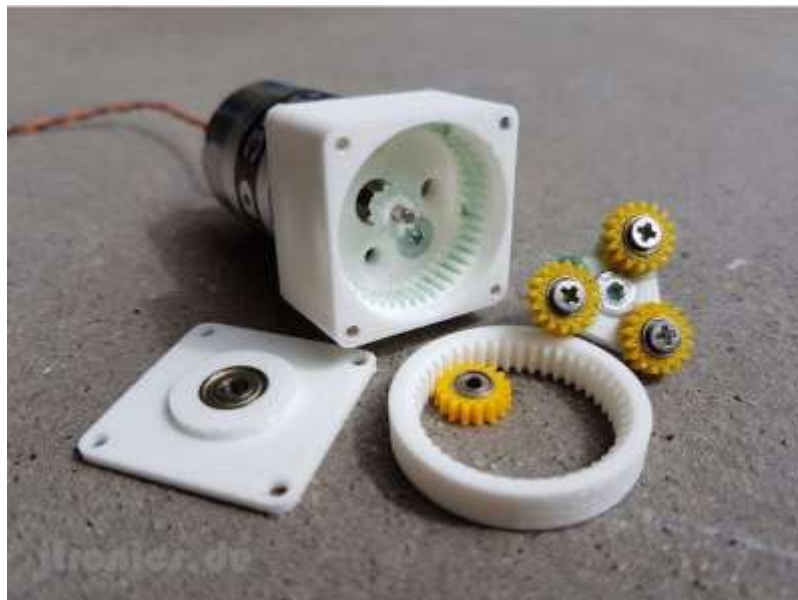
Figure 3.30 - Assembled 3D printed planetary gear reduction drive by user Jtronics
