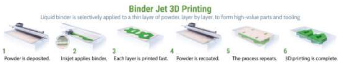
Figure 2.25 - 6 Stages of Binder Jet 3D printing [42]
