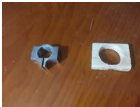
Figure 3.27 - Original metallic motor holder (left) and prototype wood motor holder (right)
