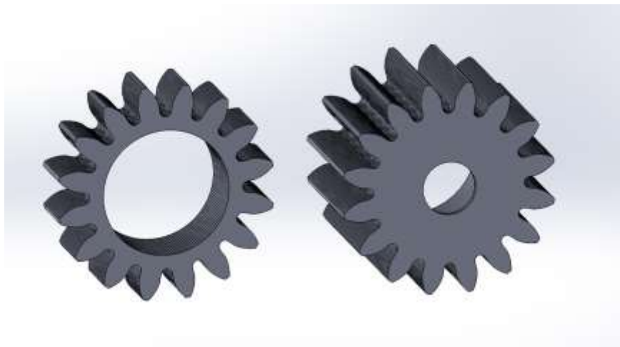
Figure 3.31 - Original planetary gear (Left) and redesigned planetary gear (Right)
