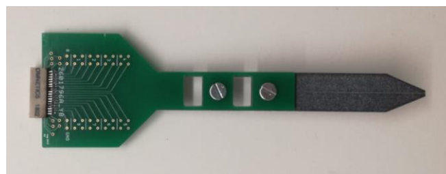
Figure 40 – Final tetrode prototype with the Omnetics connector.
