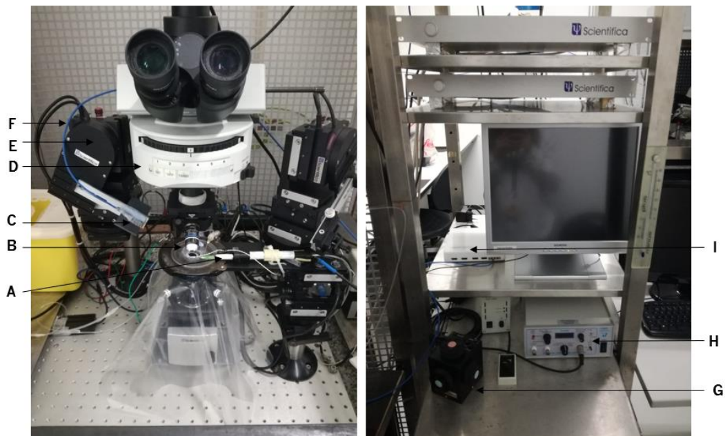
Figure 21 - Extracellular recordings' setup. (A) – in-line solution heater and cooler. (B) – recording chamber. (C) – 32-channels headstage. (D) – microscope. (E) – 3-axis micromanipulator, (F) – SPI cable, (G) – 3-axis micromanipulator control cube. (H) - automated temperature controller. (I) – Open Ephys acquisition board.
