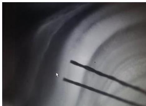
Figure 35 – Positioning of two tetrodes during the measurement of spontaneous activity in brain hippocampal slices (image obtained with the recording set up's microscope).
