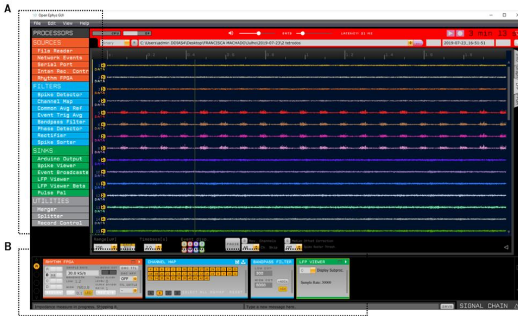
Figure 22 – Open Ephys GUI. (A) – data processing modules (“Sources”, “Filters”, “Sinks”, “Utilities”). (B) – processing pipeline.
