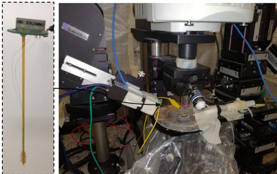
Figure 37 – Electrophysiology recordings setup using the first extracellular recording prototype for brain slices based on tetrodes.
