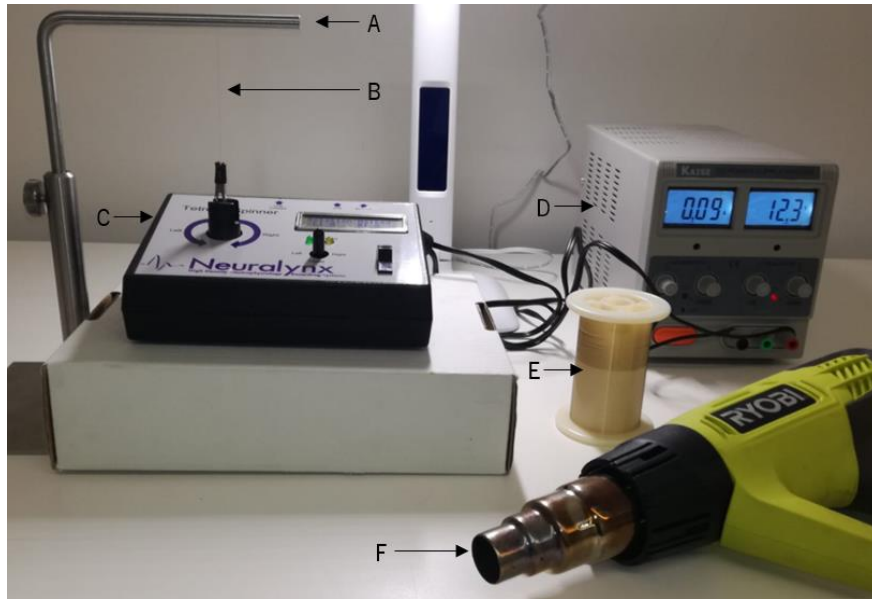
Figure 24 – Tetrode fabrication setup. (A) – horizontal metal bar. (B) – tetrode. (C) – tetrode spinner. (D) – power supply. (E) – 12.5 \mu\text{m} nichrome wire. (F) – heat gun.
