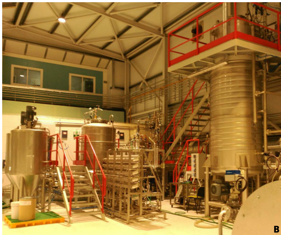
Figure 10 Industrial fermenters with a working volume of 200 L (A) and 5000 L (B). The facilities are located at Algafarm (Pataias, Alcobaça).
