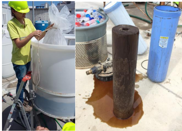
Figure 12 On the right the solubilization tank with the net inside. On the left: the filter of 20 \mu\text{m} used.
