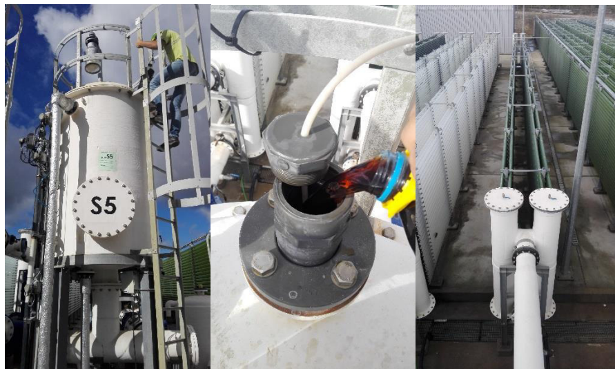
Figure 14 Addition of biological medium to an industrial PBR (10000 L)
